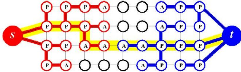
Figure 2.2: Example search tree of algorithm given in [2] at the end of growth stage.
