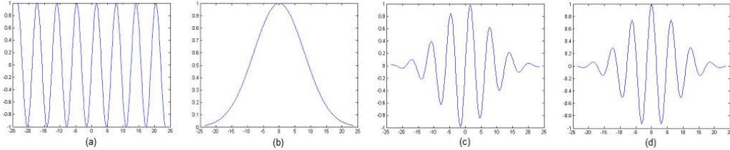
Figure 3.4: 1D composition of a Gabor filter a) A sinusoid b) A Gaussian c) Resulting Gabor filter(real part) d) Resulting Gabor filter(imaginary part)
