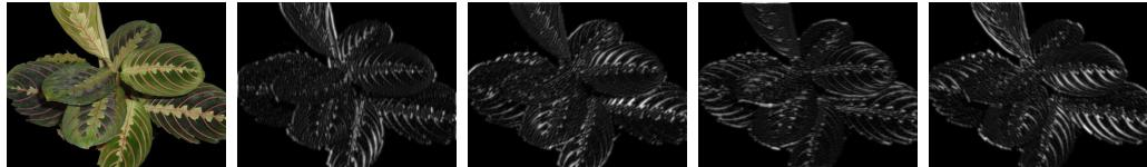
Figure 3.6: The original image and four different maps show the texture energy in different orientations (0, 45, 90, 135 from vertical, from left to right). Note that the texture in different leaves of this plant are captured in different orientations.
