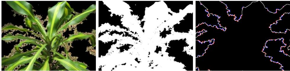
Figure 3.13: Example for a jaggy (noisy) plant contour caused by insufficient segmentation. Left: Segmented image, Middle: Segmentation map to see the segmentation faults, Right: Traced contour of the image with convex and concave points marked as blue and red, respectively
