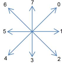
Figure 3.8: 8-directions that are used in the chain code and their corresponding enumerators
