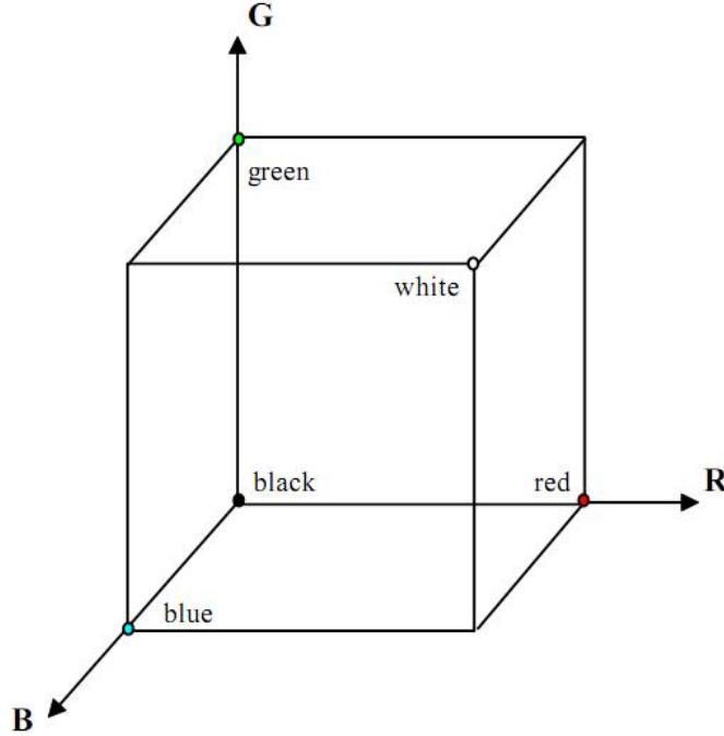
Figure 3.2: 3D RGB cube: illustrating RGB color space. Any color can be represented as a point in the color cube by (R, G, B). For example, red is (255, 0, 0), green is (0,255,0), and blue is (0, 0, 255).
