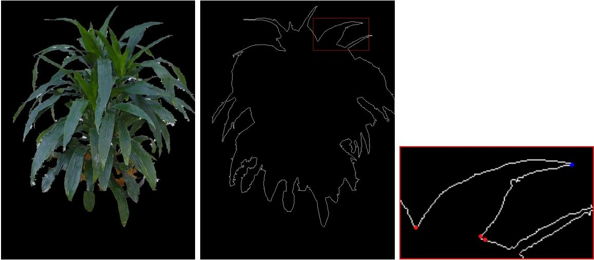
Figure 3.9: An example for contour tracing. Left: Original segmented image where background pixel value of 0 while foreground is non-zero, Center: traced contour of the image, Right: Detailed view of the contour focused on the marked region where concave and convex points are marked as red and blue.
