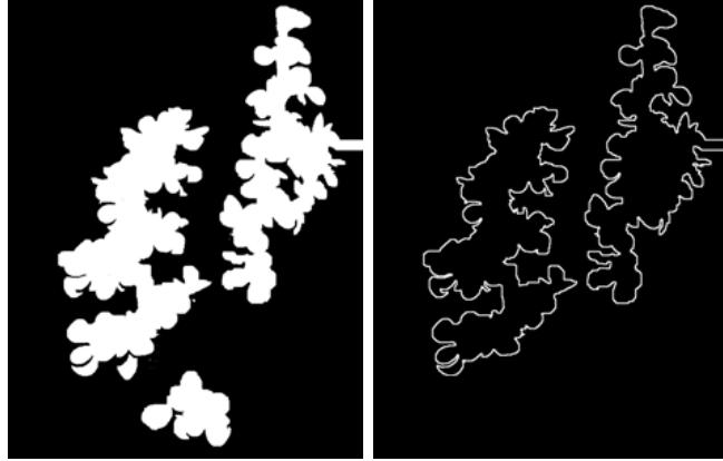
Figure 3.14: Example of a segmented plant image with three separate plant regions and its corresponding plant contour. By a small modification on contour tracing algorithm, two regions are retrieved and added to the contour.
