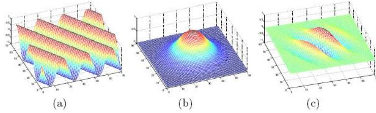
Figure 3.5: 2D composition of a Gabor filter (taken from [3]) a) A sinusoid b) A Gaussian c) Resulting 2D Gabor filter(wavelet)
