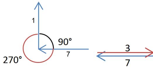
Figure 3.10: Illustration of direction change in the contour. Left: Example for wide-acute angle comparison. Direction change from 1 to 7 gives sharpness measure 2 ( $\text{abs}(1-7)=6\equiv2$ ). Right: The highest sharpness is obtained when an opposite direction is followed another ( $\text{abs}(3-7)=4$ )
