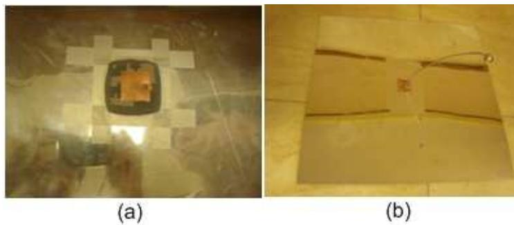
**Figure 3.18** a) Patch antenna on mosaic substrate in Figure 3.12 with b) flexible coaxial cable and aluminum ground plane
