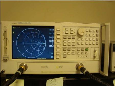
**Figure 4.36** Agilent 8720ES Network Analyzer
