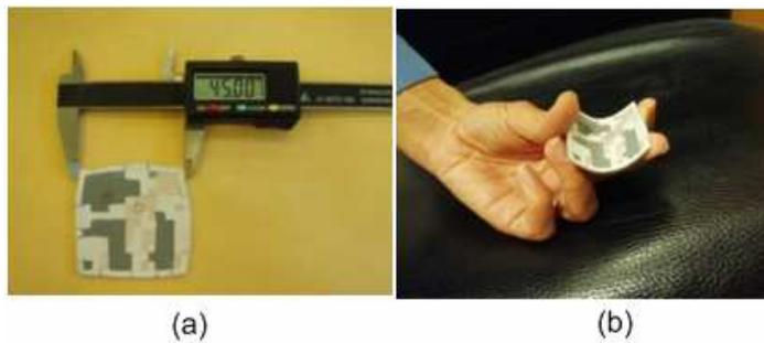
**Figure 3.10** a) 2D spatially variable flexible substrate made of MCT 20, MCT70, b) MCT15 by the dice and assembly method.
