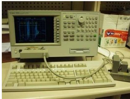
**Figure 3.7** Agilent 16451B impedance analyzer
