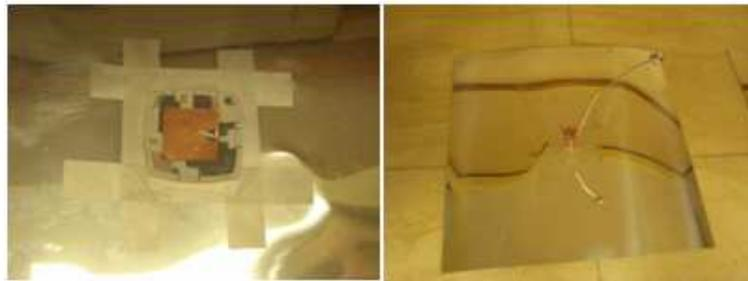
**Figure 4.30** Antenna on substrate in Figure 3.10 fabricated using the dice and assembly method
