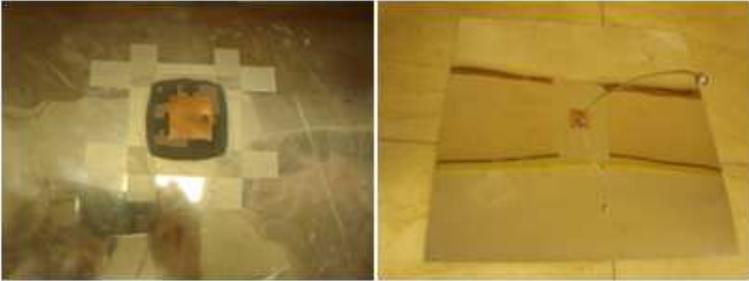
**Figure 4.33** Antenna on substrate in Figure 3.11 fabricated using the second fabrication method
