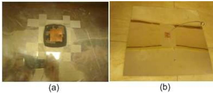
**Figure 3.18** a) Patch antenna on mosaic substrate in Figure 3.12 with b) flexible coaxial cable and aluminum ground plane
