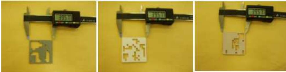
**Figure 3.11** Machined mosaic substrates which are made from MCT70 (left), MCT20 (center) and MCT15 (right) ceramic-polymer tapes.
