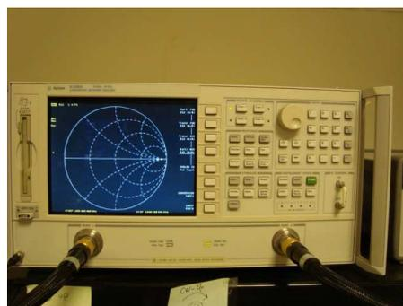
**Figure 4.36** Agilent 8720ES Network Analyzer
