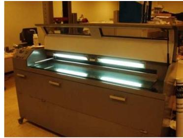
**Figure 3.3** Tape casting process
