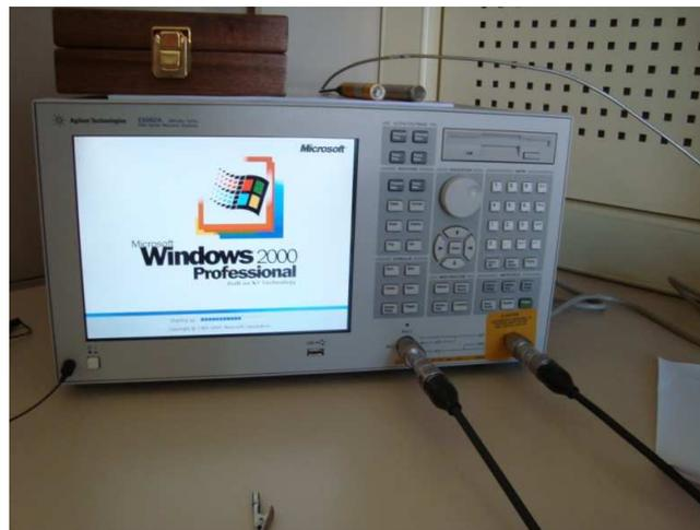
**Figure 3.20** Agilent E5062A Series Network Analyzer
