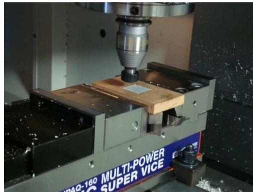
**Figure 3.1** Hole drilling process within the substrate using CNC
