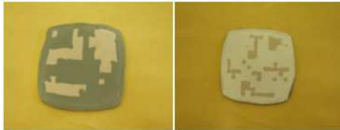
**Figure 3.12** Resulting 3D spatially variable substrates after pressing three machined material layers with different dielectric constant and material layout (as shown in Figure 3.11)
