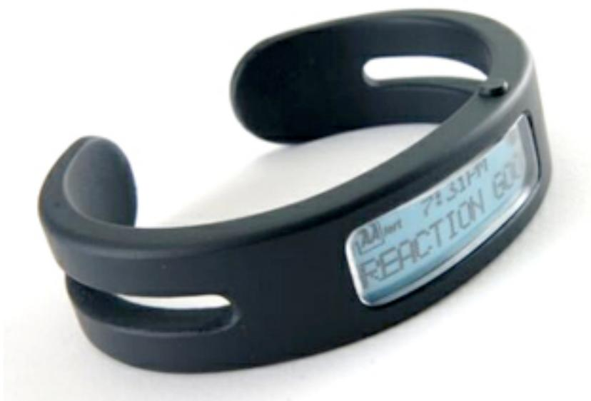
Figure 2.1: AAlert wristband driver drowsiness detection device developed by Dan Ruffle. The device uses motion combined with reaction time to determine whether or not the driver is in a drowsy state.
