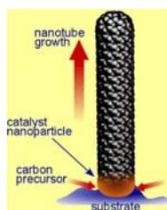
**Figure 1.** Schematic representation of CNT growth on the metal incorporated MCM-41 mesoporous molecular substrate
