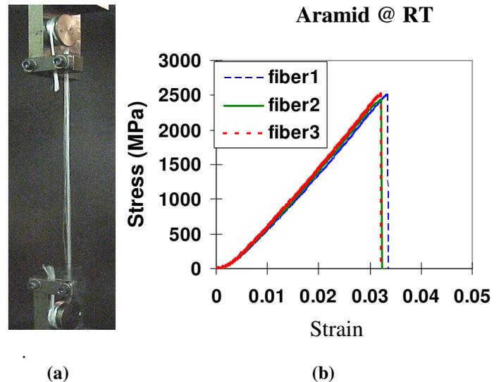
Fig. 1 Tensile tests: a) configuration b) repeatability.
