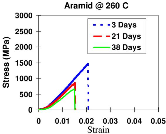
Fig. 3 Fiber strength upon exposure to 260 °C (500 °F).
