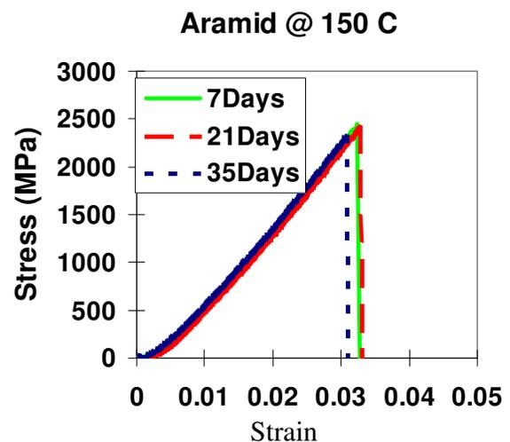
Fig. 2 Fiber strength upon exposure to 150 °C (302 °F).
