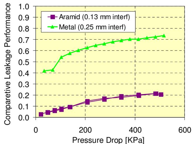
**Fig. 8** Sample Aramid Seal Leakage Data
