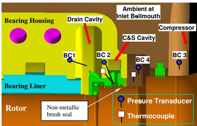
**Fig. 9** The 7EA #1 (inlet) bearing sealing application
