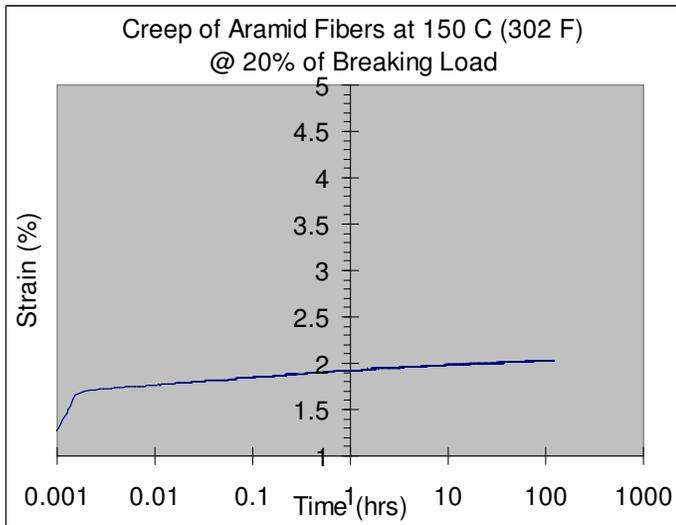
Fig. 4 Creep strength at 150 °C (302 °F).
