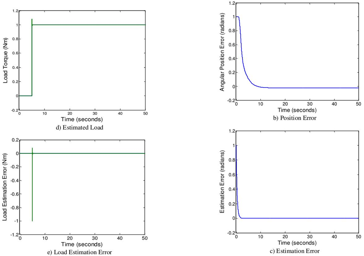
Fig. 7: a) Position output, b) Angular position error, c) Estimation error, d) Estimated load torque (EKF), and e) Load estimation error of system under constant load, and simultaneously applied *random* control delay and *random* measurement delay (1-2 sec) with PD+ controller, SMO and EKF observer.
