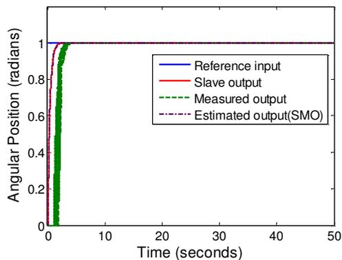
Fig. 6: Position output of system under constant load and random measurement delay (1-2 sec) with PD+ controller, SMO and EKF observer.
