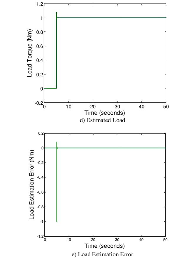
Fig. 9: a) Position output, b) Angular position error, c) Estimation error, d) Estimated load torque (EKF), and e) Load estimation error of system under constant load, random control delay and measurement delay (1-2 sec) with and doubled viscous friction ( $B$ ) with PD+ controller, SMO and EKF observer.
