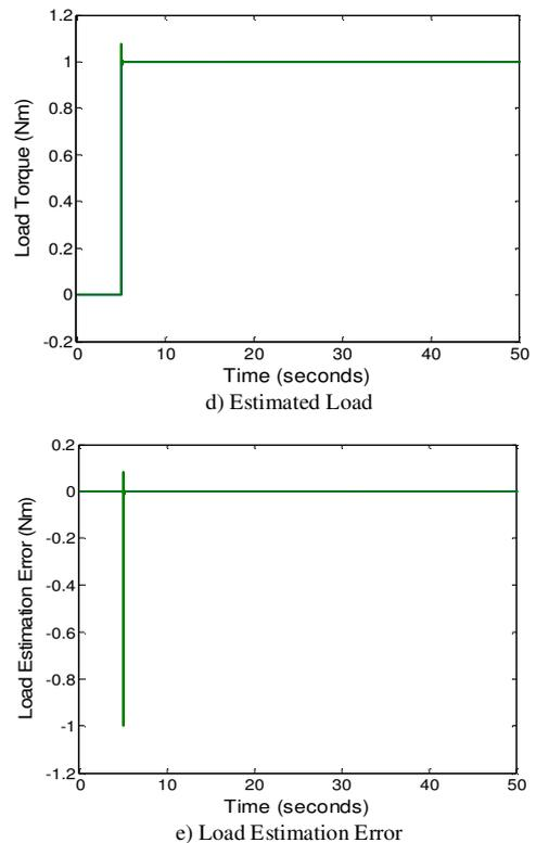
Fig. 8: a) Position output, b) Angular position error, c) Estimation error, d) Estimated load torque (EKF), and e) Load estimation error of system under constant load, random control delay and measurement delay (1-2 sec) with inertial variation ( $J = 2*J$ ) with PD+ controller, SMO and EKF observer.
