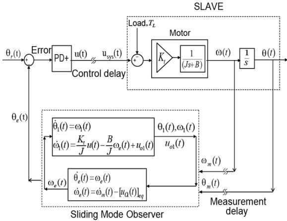
Fig. 1: Block diagram of system with SMO compensating measurement delay.
