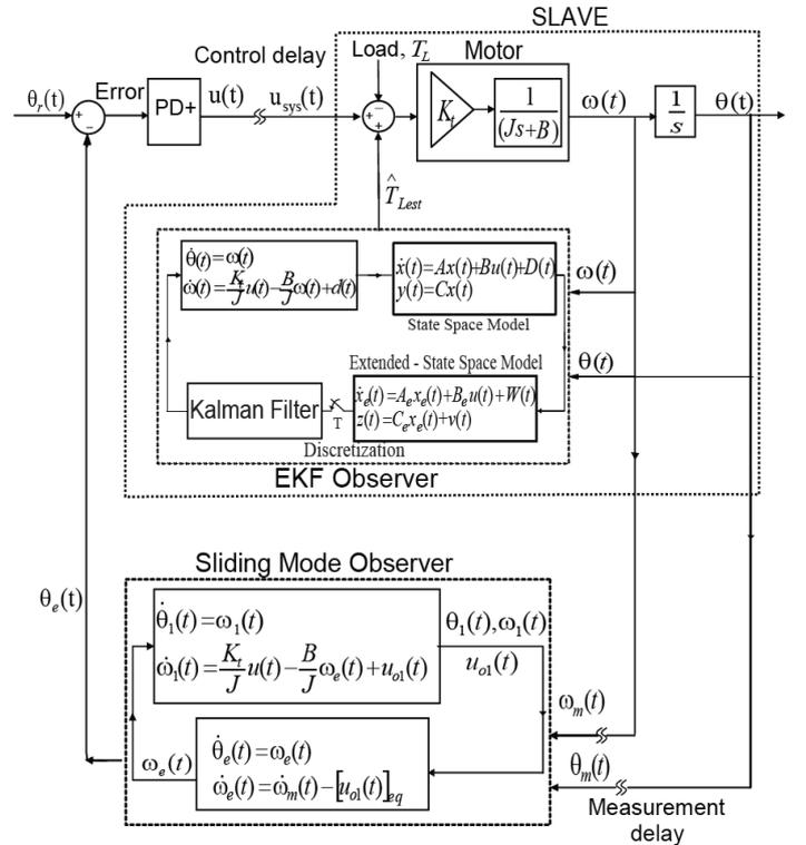
Fig. 2: Block diagram of the full system with PD+, SM and EKF observers.
