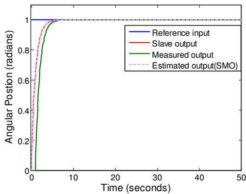
Fig. 5: Position output of system under a constant load and constant measurement delay (1 sec), with PD+ controller and EKF.
