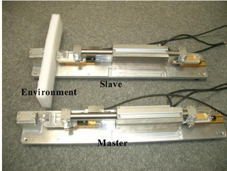
Fig. 11. The bilateral master/slave robots
