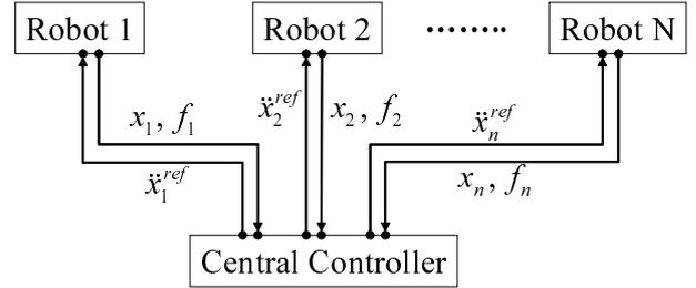
Fig. 4. The proposed structure for a hybrid control system with multiple plants
