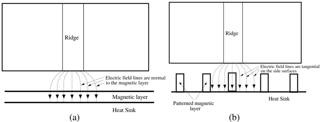
**Figure 4.** (a) Continuous recording medium is illustrated in the vicinity of a ridge waveguide. The electric field lines are normal to the continuous recording medium. (b) The electric field lines are both normal (at the top surfaces) and tangential (on the side surfaces) to the patterned media.
