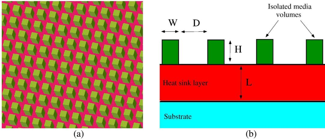
**Figure 2.** (a) An oblique view of the patterned magnetic medium with optically and thermally isolated magnetic particles placed over a heat sink layer, (b) Patterned magnetic medium with optically and thermally isolated magnetic particles placed over a heat sink layer. The geometric dimensions of the particle size and separation as well as the thicknesses of the magnetic and heat sink layers are shown.
