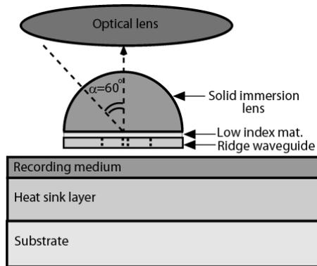
**Figure 1.** A schematic illustration of an optical transducer, which is placed at the end of an optical lens system, is given. The optical transducer is placed in the vicinity of a near-field sample, which is the recording magnetic medium for HAMR.
