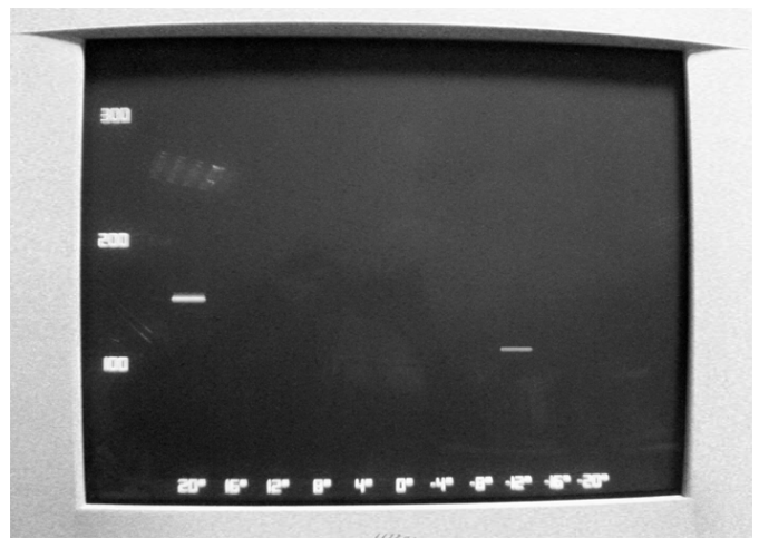
Fig. 6. Experiment-II. A good reflector is placed 150 cm away from the device with an angle of 20^\circ . A bad reflector is placed 120 cm away from the device with an angle of -12^\circ . The good reflector appears brighter and the bad reflector appears dimmer in the image. The image has 21 dB dynamic range.
