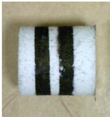
Figure 20 : Gold-electroded tubular PVDF electrospun mat specimen used for in-plane strain measurements.
