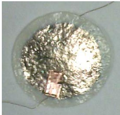
Figure 11 : ZnO/PVDF nanopowder composite pressed into a pellet.
