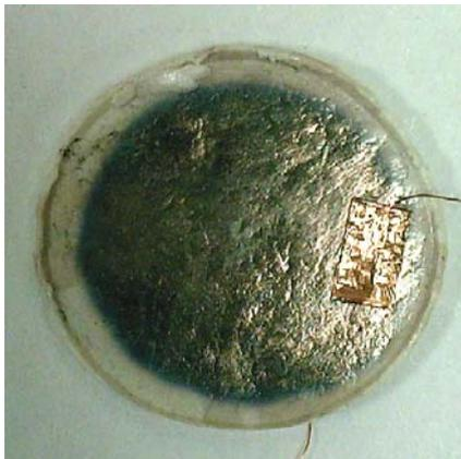
Figure 10 : ZnO fiber mat sandwiched in between two PVDF fiber mats.
