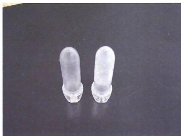
Figure 24: Opacity noted following oxidation
