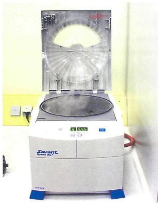
Figure 16: Preheated speedvac showing humid atmosphere used to minimize evaporation from tubes.
