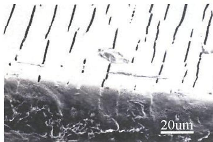
Figure 26: SEM micrograph of APS-treated, oven-heated tube taken from the cross-sectional viewpoint but tilted slightly towards the inner face.
