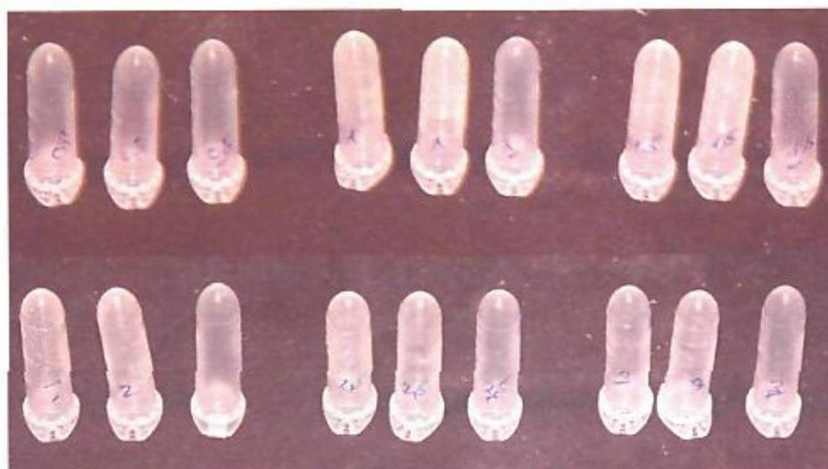
Figure 20: Photograph showing the optical effect of the oxidation caused by different concentrations of persulfates during the concentration course (Sets of tubes from left to right and top to bottom: 0.5M APS; 1M APS; 1.5M APS; 2M APS; 2.5M APS; and 3M APS).
