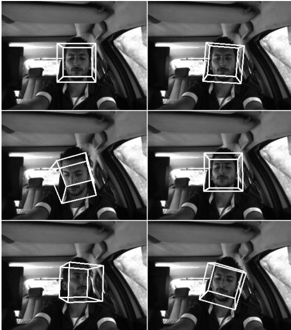
Fig. 1. Result of the driver head tracker at frames: 0, 60, 110, 150, 230, 400
