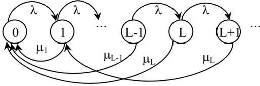
Figure 3: Markov-chain representation of aggregate frame transmission
