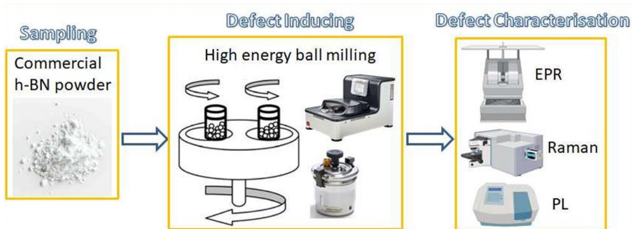
Figure 3: Schematic of the sampling, defect inducing, and defect characterization of intrinsically defective h-BN
