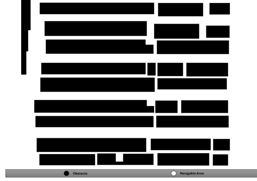
(b) A formatted approximation of the Ambarli Port map, prepared to be compatible with the proposed algorithms for conducting multi-goal path planning tasks.
