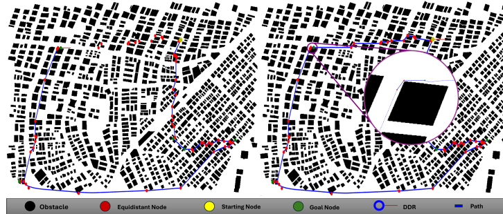
(c) An image that illustrates a trajectory followed by a three-wheeled omnidirectional robot. The left side shows the simulated robot navigating the given path, indicating its position. The right side displays the complete trajectory after navigation, highlighting control behaviours used for sharp turns.
