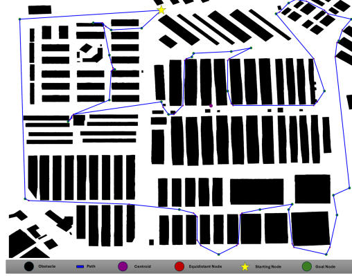
(b) Illustrative solution for a randomly distributed set of goal nodes within the Ikitelli Sanayi industrial area.
