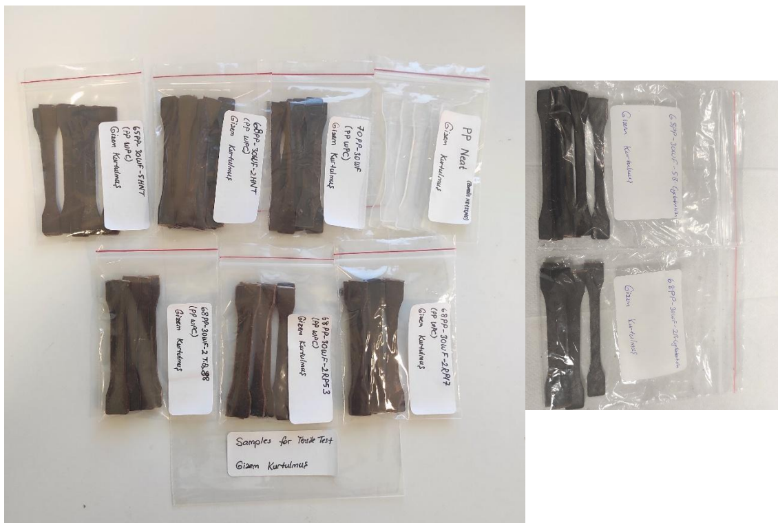
Figure 3. Injection molded samples that composed of 2 wt.% and 5 wt.% HNT, \beta -CD, and 2 wt.% commercial additives
