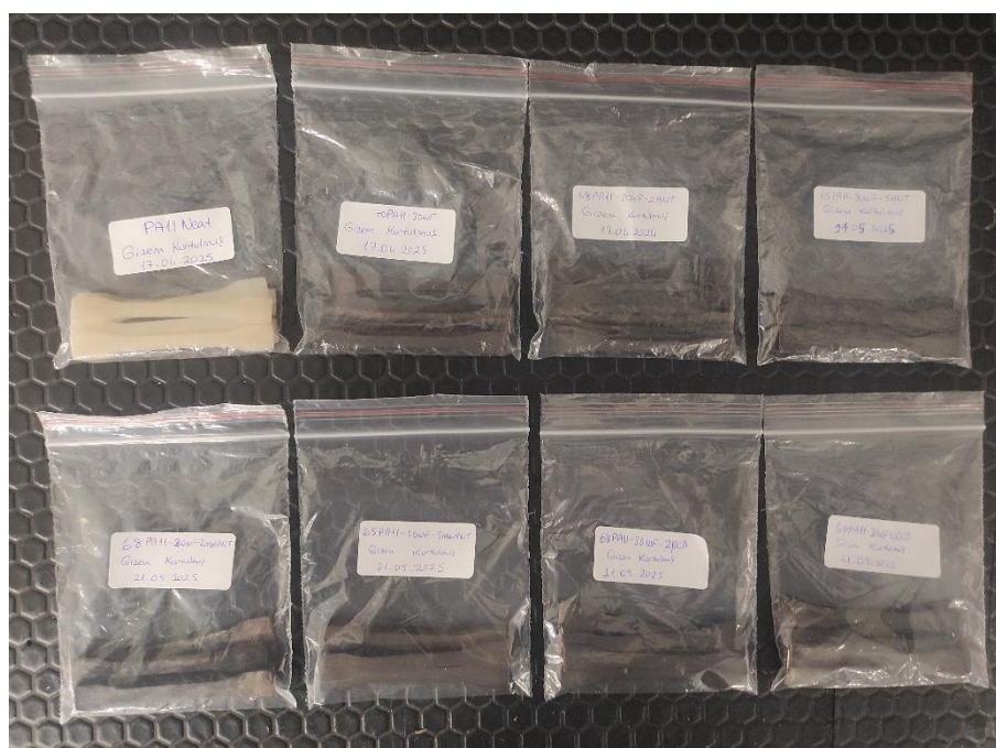
Figure 25. Injection molded PA11-based WPC samples with HNT, Mod-HNT and \beta -CD
