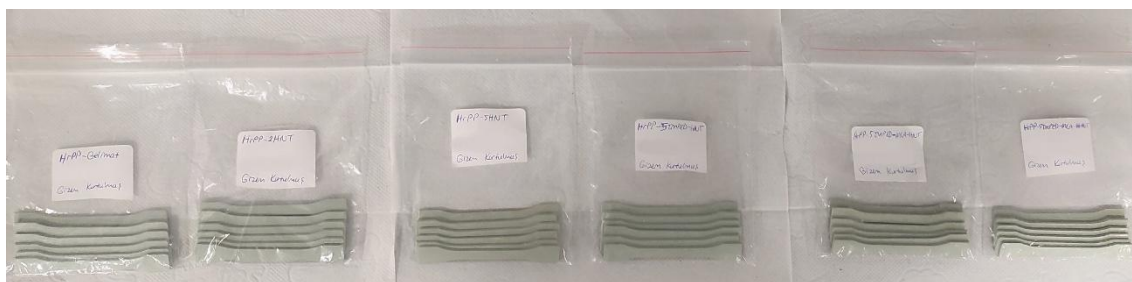
Figure 14. Samples formed by molding the granules in the injection device to be used in the tests: rPO-Neat, rPO-2HNT, rPO-5HNT, rPO-5TMPED-HNT, rPO-5TMPED-MCA-HNT, rPO-5TMPED-MCA-HH-HNT
