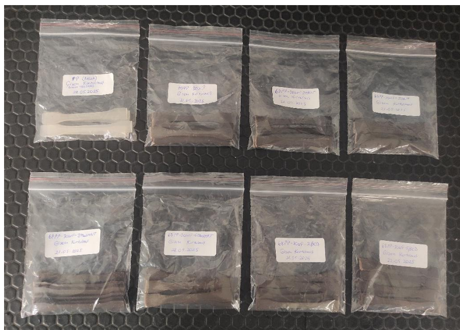
Figure 24. Injection molded PP-based WPC samples with HNT, Mod-HNT and \beta -CD
