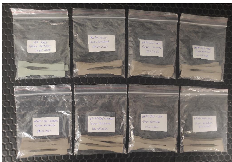
Figure 23. Injection molded rPO-based WPC samples with HNT, Mod-HNT and \beta -CD
