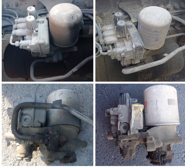
Figure 1.4 Service images of failed E-APU units (Mumcuoglu et al., 2024b), shown both installed and removed examples, illustrating progressive wear and operational damage.
