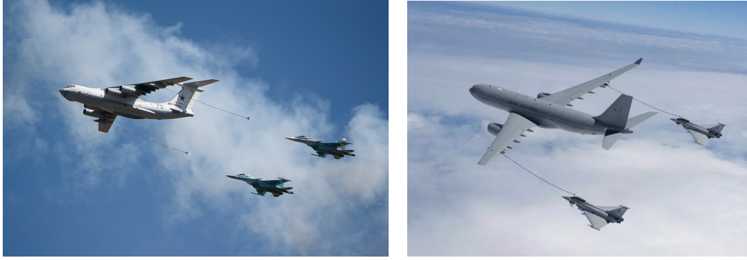
Figure 1.4 Simultaneous aerial refueling with multiple receivers (Quantity & of russian Il-78 [Online image], air; for energy efficient inter-UAV collision avoidance, rus)
