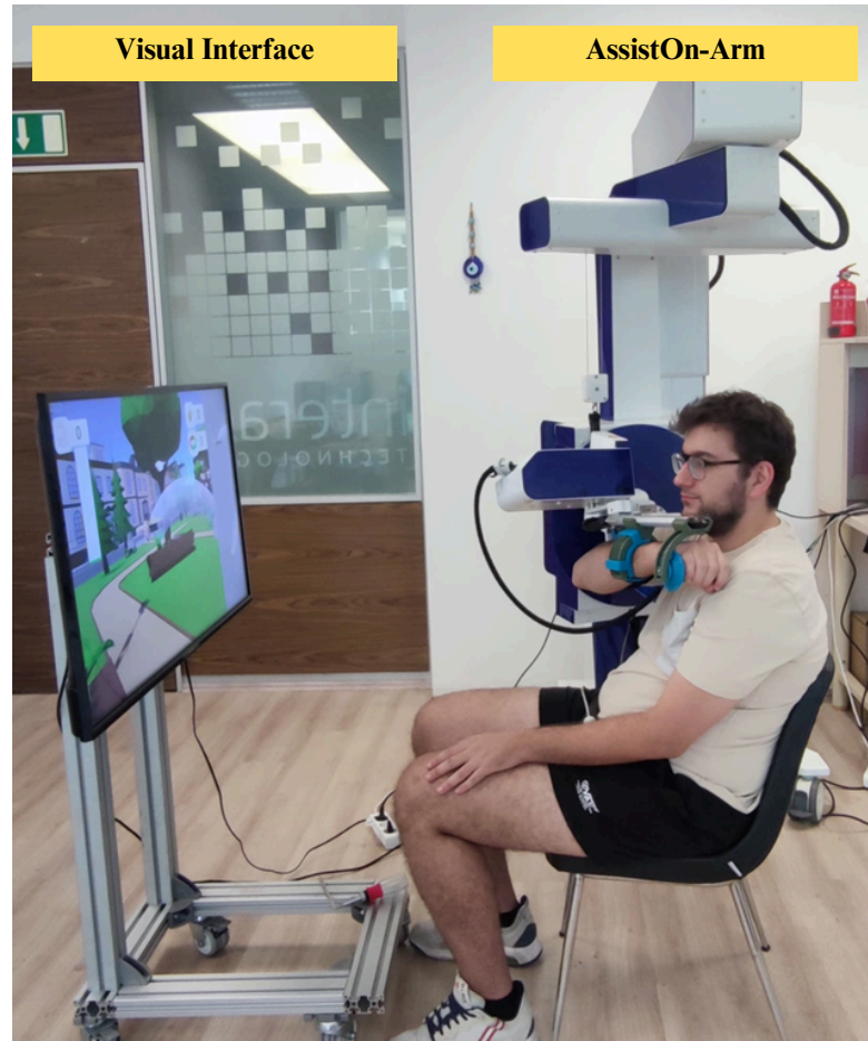
FIGURE 6.4: Experimental setup including a visual display and assistive rehabilitation robot, AssistOn-Arm
