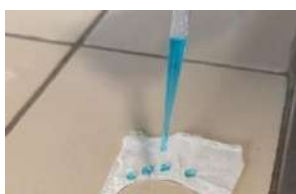
Figure 3.3.1: A blue water droplet remains on the PAN/F-SiO 2 membrane, showing enhanced hydrophobicity.
