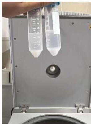
Figure 2.4.1: Image of the solution after centrifugation: the upper clear liquid is the supernatant, and the white sediment at the bottom represents the fluorine-modified SiO 2 (F-SiO 2 ) nanoparticles.
