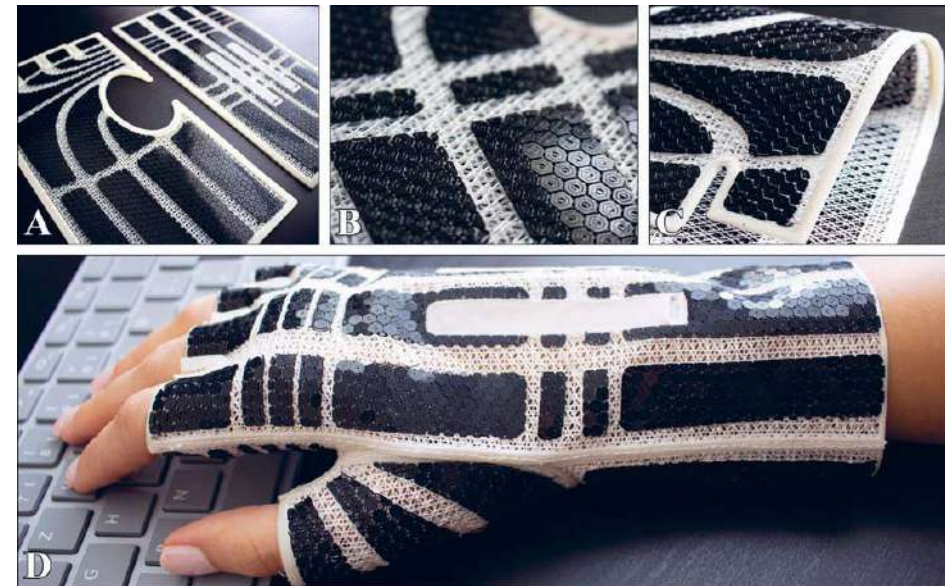
3D printed glove: A) sewing pattern printed from two materials, B) surface design of glove, C) flexible sewing pattern with inner lining, D) pattern pieces sewn together to form three-dimensional garment
