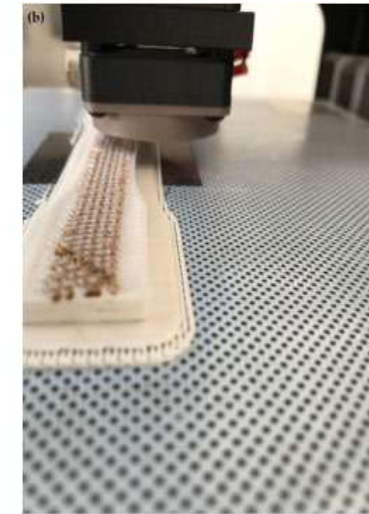
Photographs and schematic representations of: (a) jute fabrics, (b) 3D printing on jute fabric
