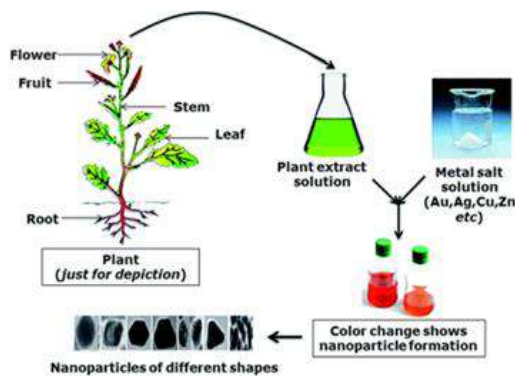
Figure 1. Preparation of solution from plant extract and production of nanoparticles by green synthesis.
