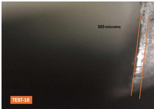
Figure 26: Wear status of Tool-life optimized result
