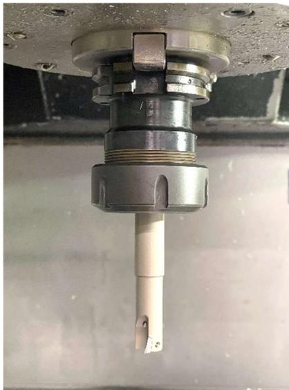
Figure 19: The cutting tool on machining center
