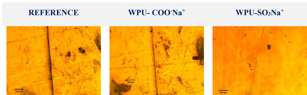
Figure 21: Optical microscope images for self-healing for different ionic groups
