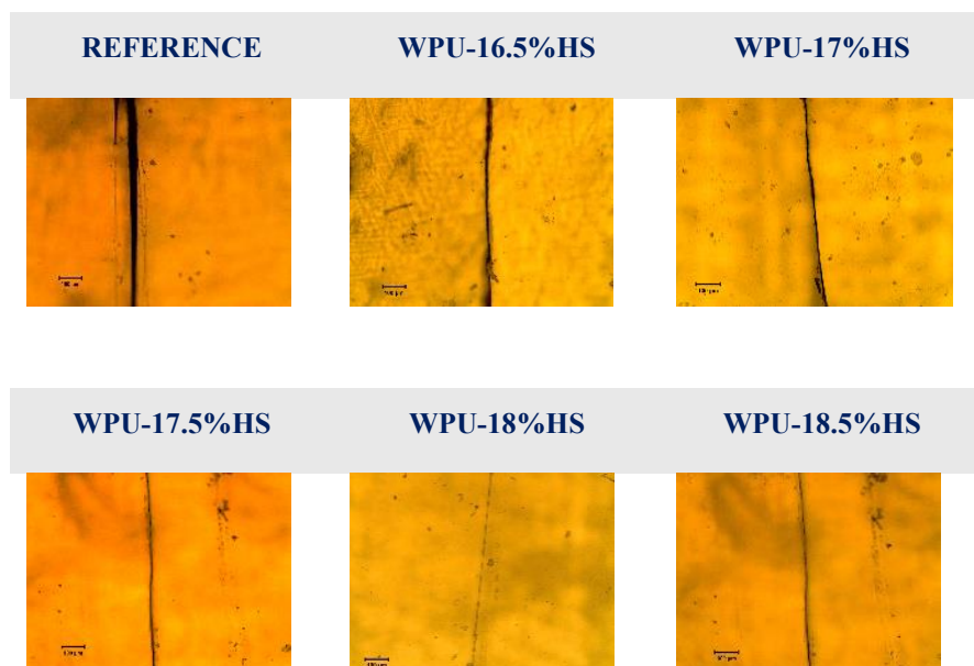
Figure 19: Optical microscope images of PU films for self-healing at different hard segment contents
