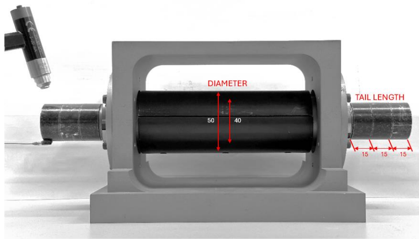
Figure 16: Experimental setup for tail length sensitivity analysis
