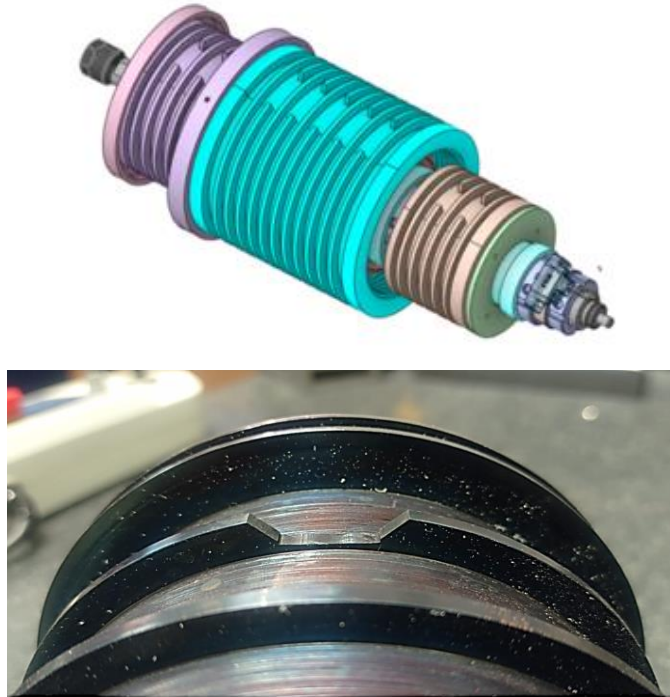
Figure 48: Motor cooling jacket design
