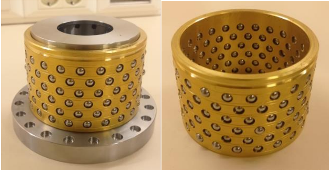
Figure 41: Ball cage mechanism for constant preloading system
