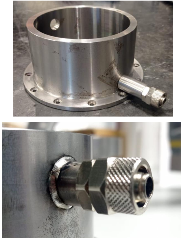
Figure 52: Mechanical connectors for cooling water supply
