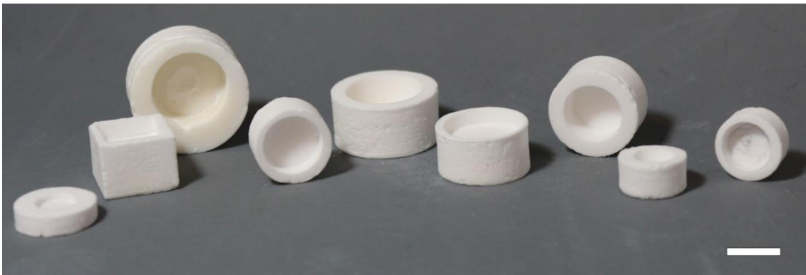
Figure 2.24 House-made alumina crucibles with varying dimensions, scale bar represents 1 cm.
