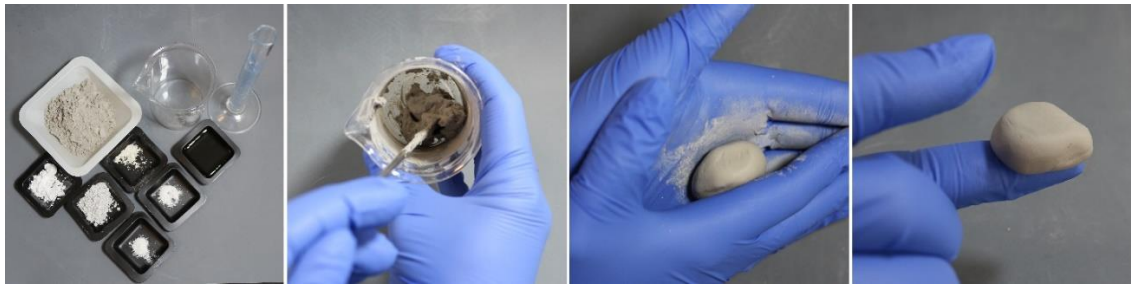
Figure 3.2 The steps involved in preparing a self-standing dough consisting of 72.7 wt. % SiAlON and 2 wt. % copolymer.
