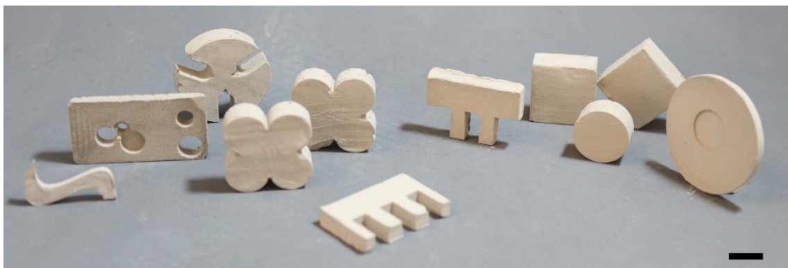
Figure 3.9 Custom-sized shapes at their green state after machining (Scale bar represents 1 cm.)
