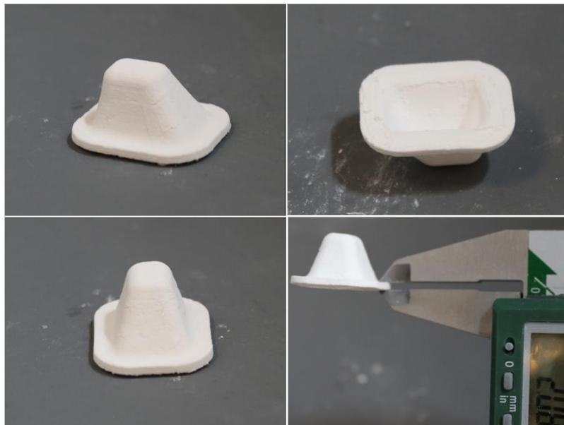
Figure 2.25 A complex, curvy-shaped alumina body having a 2 mm wall thickness
