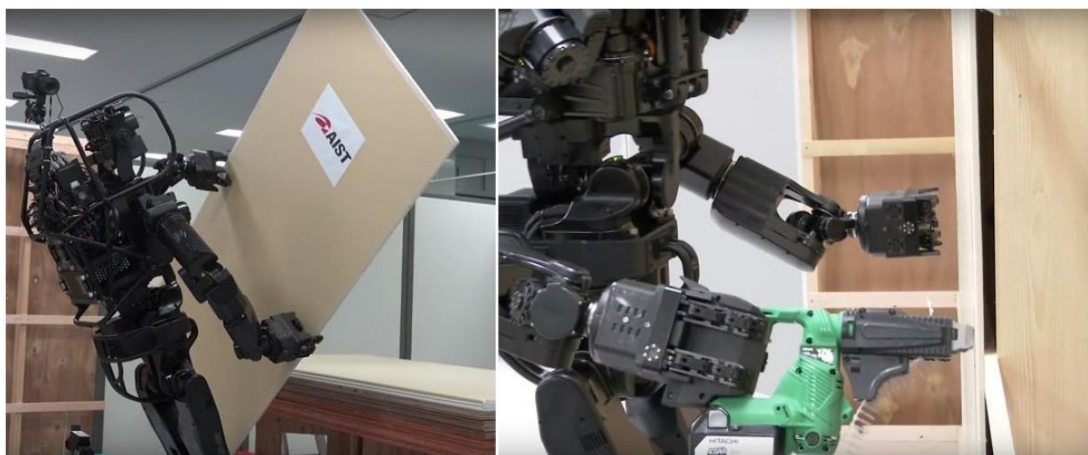
Figure 2. 11 Images of HRP-5P performing simple but heavy-duty constructions tasks (ARCH2O HRP-5P, 2024)
