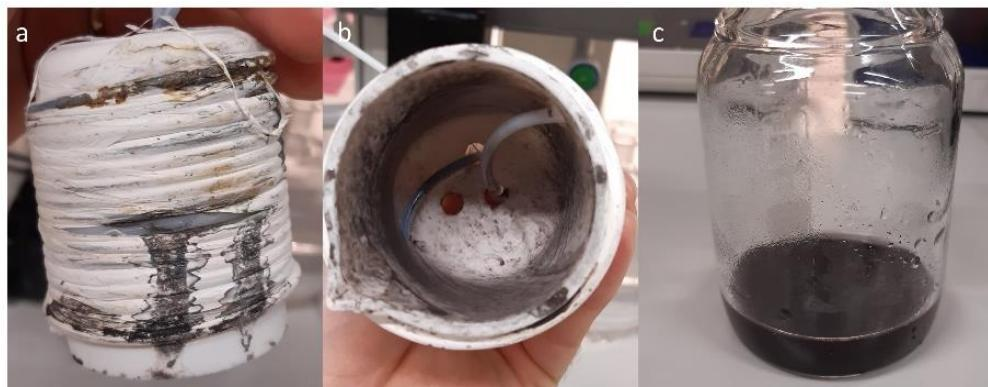
**Figure 4-6:** Images of (a),(b) blockage, happened, (c) precipitation formed.
