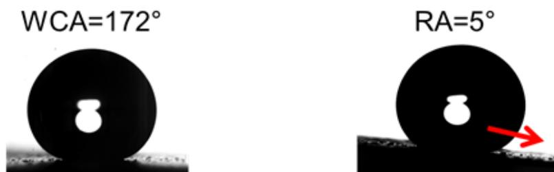
Figure 18. Contact angle and contact angle hysteresis measurements of ZIF-8 based coating.
