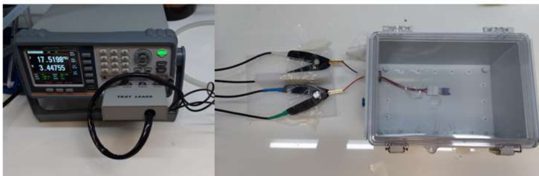
Figure 8 Gas sensor characterization setup connected to an LCR meter.
