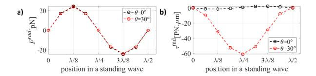
Fig 3.2. The radiation force and torque with respect to  $\Delta z$  in a standing wave on a horizontal ( $\theta = 0^{\circ}$ ) and tilted ( $\theta = 30^{\circ}$ ) polystyrene ring in a viscous water for f = 2 MHz. a)  $F^{rad}$  and b)  $\tau^{rad}$  profiles.
