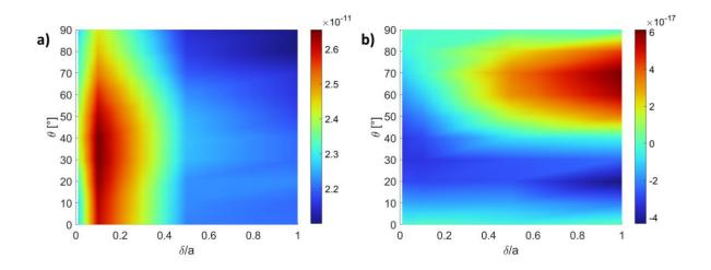
Fig 3.8 The change of (a)  $F^{rad}$  and (b)  $\tau^{rad}$  with respect to  $\theta - \delta/a$ . The standing field is applied in the z-direction on a polystyrene ring in a viscous fluid with different viscosities when  $\theta$  varies between 0° and 90°.
