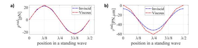
Fig 3.3. a) Comparison of the acoustic radiation forces corresponding to inviscid and viscous fluids b) Acoustic radiation torque comparison of viscous and inviscid fluids.
