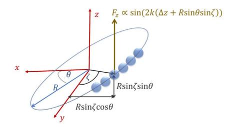
Fig. A1. Representation of the local acoustic radiation force on a tilted ring, which is approximated by a chain of spherical particles.
