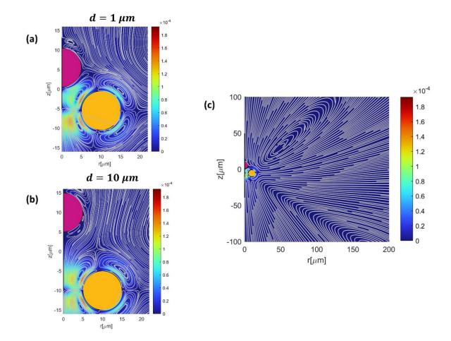
Fig 4.14. Streamline patterns for polystyrene sphere and copper ring in water subjected to a standing wave at f = 500 KHz at different inter-distances: a)  $d = 1 \mu m$  b)  $d = 10 \mu m$  c)  $d = 1 \mu m$ ; first particle is a ring with  $a = 5 \mu m$  and  $R = 10 \mu m$ , and second particle is a sphere with the radius of  $a = 5 \mu m$ .
