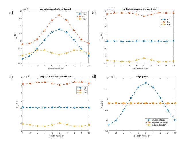
Fig 4.4. Local acoustic radiation forces (ARF) on each segment of polystyrene and contribution of pressure and velocity terms to ARF for f = 0.6MHz; (a) the forces on the complete ring composed of segments in contact, (b) forces on the detached segments forming a ring (c) forces on each individual segment placed in the acoustic field without others (see the picture in Fig.4.3a).
