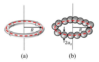
Fig 4.1. Schematic of chain-of-spheres methodology. (a) Shows the original ring geometry, (b) shows the representation of the ring with  $N_{sph} = 14$  spheres with radius  $a_s$  placed along the circle of the ring which is *R* away from the center of the ring. The circle is shown in red dashes.
