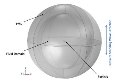
Fig 2.2. Viscous Simulation domain with the ring placed inside a fluidic domain with PML, nonreflecting radiation conditions at the boundaries.
