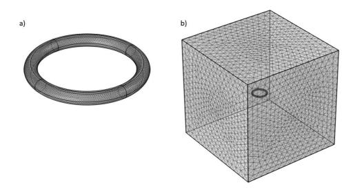
Fig 2.4. Mesh on a) a ring particle, b) fluid domain.
