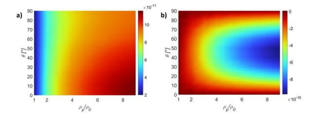
Fig 3.9 The change of (a)  $F^{rad}$  and (b)  $\tau^{rad}$  with respect to  $\theta - \rho_p / \rho_0$ . The standing field is applied in the z-direction in a viscous fluid with different densities for the ring when  $\theta$  varies between 0° and 90° at  $\Delta z = \lambda/8$ .
