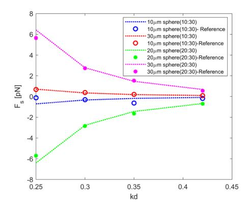
Fig 2.8.The comparison of the secondary forces between spheres (sphere1: sphere2). Dashed lines are the simulation results, datapoints are from Hoque and Sen (Hoque & Sen, 2020).
