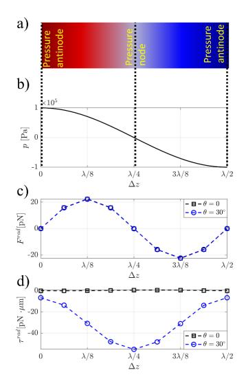
Fig 3.1. The radiation force and torque with respect to  $\Delta z$  in a standing wave on a horizontal ( $\theta = 0^{\circ}$ ) and tilted ( $\theta = 30^{\circ}$ ) polystyrene ring in water for a f = 2 MHz. a) Color plot of the pressure amplitude, b) Change of p with respect to  $\Delta z$  and the corresponding c)  $F^{rad}$  and d)  $\tau^{rad}$  profiles.
