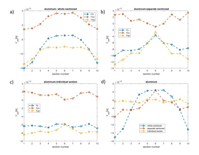
Fig 4.5. Local acoustic radiation forces (ARF) on each segment of aluminum ring and contribution of pressure and velocity terms to ARF; (a) the forces on the complete ring composed of segments in contact, (b) forces on the detached segments forming a ring (c) forces on each individual segment placed in the acoustic field without others (see the picture in Fig. 4.3a).
