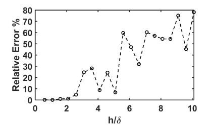
Fig 2.6. Mesh convergence studies with respect to the maximum element size.
