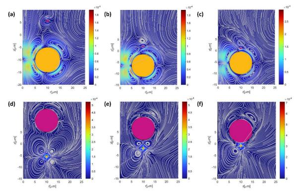
Fig 4.10. Streaming patterns and second-order velocity field are shown for polystyrene and copper rings at f = 500 KHz and  $R = 10 \mu m$  with various inter-distances,  $d = 10,3,1 \mu m$  respectively (a-c) for  $a_1 = 5 \mu m$  copper,  $a_2 = 0.5 \mu m$  polysyrene, (a-c) for  $a_1 = 0.5 \mu m$  copper,  $a_2 = 5 \mu m$  polysyrene.
