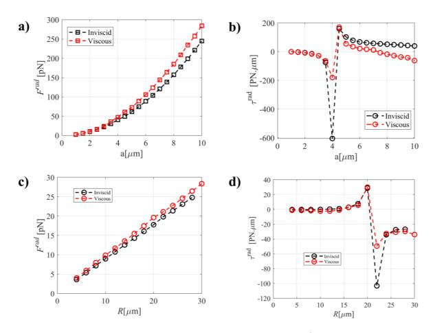
Fig 3.12. Comparison of results for viscous and inviscid fluids (a) Change of  $F^{rad}$  with respect to a, (b) change of  $\tau^{rad}$  with respect to a, (c) change of  $F^{rad}$  with respect to R and (d) Change of  $\tau^{rad}$  with respect to R.
