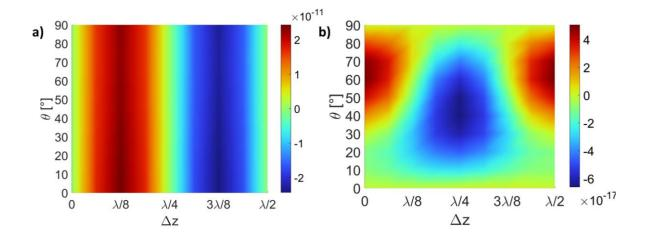
Fig 3.7 The change of (a)  $F^{rad}$  and (b)  $\tau^{rad}$  with respect to  $\theta - \Delta z$ . The standing field is applied in the z-direction on a polystyrene ring in a viscous fluid when  $\theta$  varies between 0° and 90°.
