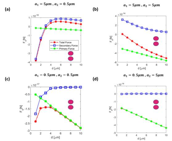
Fig 4.11. Acoustic radiation forces shown for polystyrene spheres at f = 500 KHz and reported forces are forces on the second particle.
