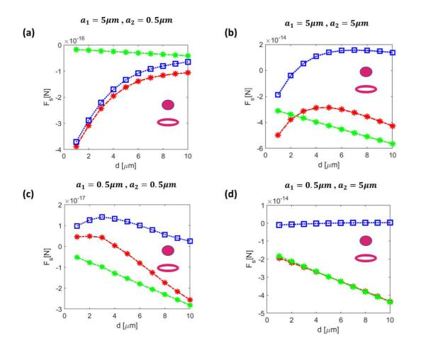
Fig 4.12. Acoustic radiation forces shown for polystyrene sphere and ring at f = 500 KHz and (first particle is ring with  $R = 10 \mu m$  and second particle is sphere): reported forces are forces on the second particle.
