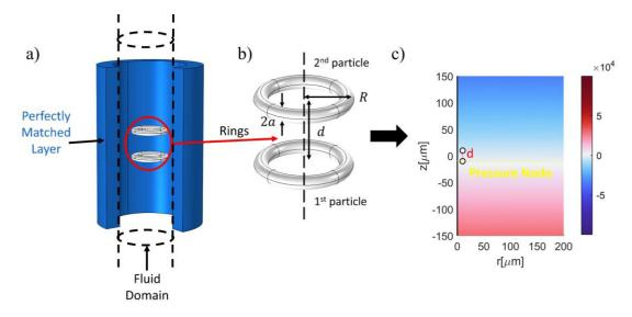
Fig 2.3. Depiction of simulated geometries. (a)-(c) show the configuration where the rings are placed along the propagation axis of the acoustic field and. (a) depict the 3-dimensional geometry, (b) show the arrangement of the rings alongside the geometric parameters and (c) show the 2-dimensional, axisymmetric domains simulated with the standing acoustic field. Note that the ring or domain dimensions are not to the scale.
