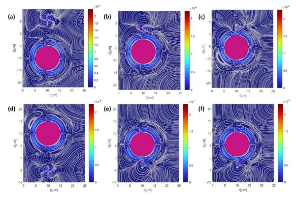
Fig 4.9. Streaming patterns and second-order velocity field are shown for polystyrene rings at f = 500KHz and  $R = 10\mu$ m with various inter-distances,  $d = 10,3,1 \mu$ m respectively (a-c) for  $a_1 = 5\mu$ m,  $a_2 = 0.5\mu$ m, (a-c) for  $a_1 = 0.5\mu$ m,  $a_2 = 5\mu$ m.
