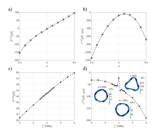
Fig 3.13. The change of (a)  $F^{rad}$  and (b)  $\tau^{rad}$  with respect to  $\phi$ . The change of (c)  $F^{rad}$  and (d)  $\tau^{rad}$  with respect to *f*. Insets show the deformations (5000 times scaled-up) and Mises stresses in the rings.
