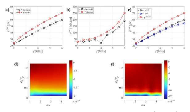
Fig 3.14. Comparison of the results of viscous and inviscid fluids; The change of (a)  $F^{rad}$  and (b)  $\tau^{rad}$  with respect to f (c) Comparison of  $F^{rad}$  with considering different contributions. The change of (d)  $F^{rad}$  and (e)  $\tau^{rad}$  with respect to  $\rho_0/\rho_p$  and  $\delta/a$ .
