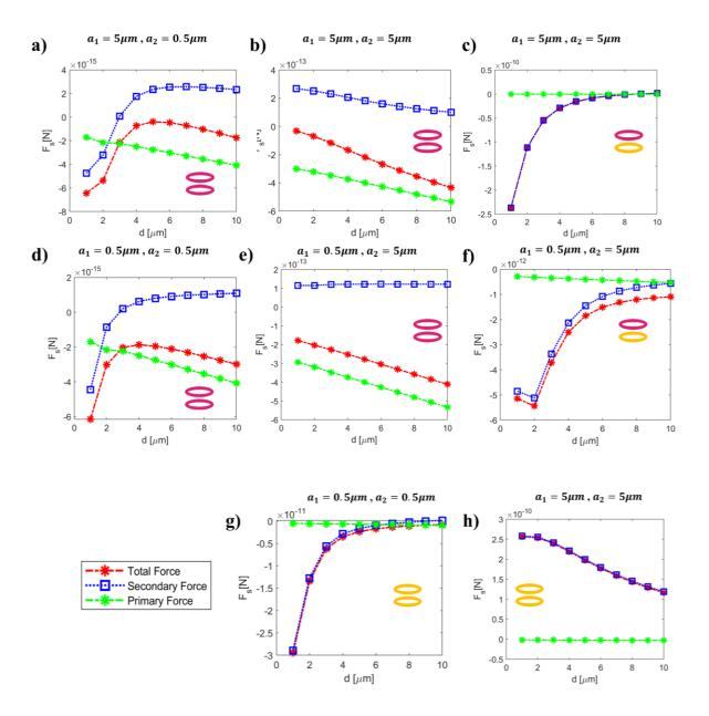
Fig 4.7. Acoustic radiation forces on particle 2 with respect to surface-to-surface distances, d,  $(1\mu m \ to \ 10 \ \mu m)$  for various sizes of the rings at f = 500 KHz and  $R = 10\mu m$  with various combination of a : (a,b,d,e) Polystyrene rings ,(c,f) First particle, a copper ring, centered at nodal plane; second particle is a polystyrene ring away from the nodal plane , (g,h) Copper rings (yellow rings represent the copper rings).
