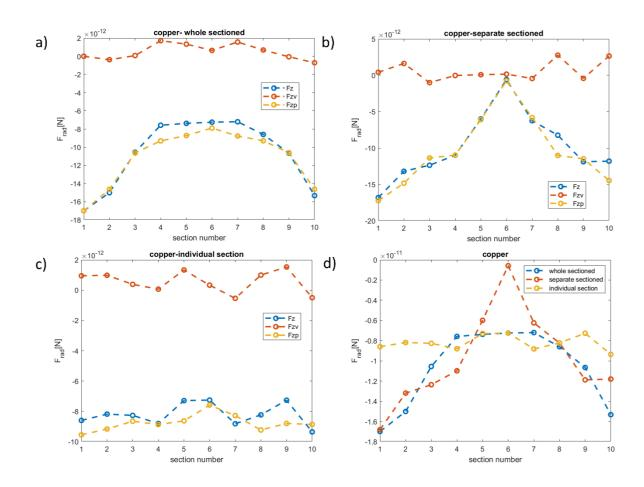
Fig 4.6. Local acoustic radiation forces (ARF) on each segment of copper ring and contribution of pressure and velocity terms to ARF; (a) forces on the complete ring composed of segments in contact; (b) forces on the detached segments forming a ring; (c) forces on each individual segment placed in the acoustic field without others (see the picture in Fig. 4.3a).
