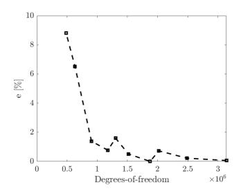
Fig 2.5. Convergence of  $F^{rad}$  with respect to the degrees of freedom.
