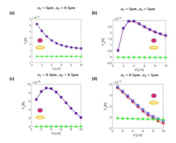
Fig 4.13. Acoustic radiation forces shown for polystyrene sphere and copper ring at f = 500 KHz and (first particle is ring with  $R = 10 \mu m$  and second particle is sphere).
