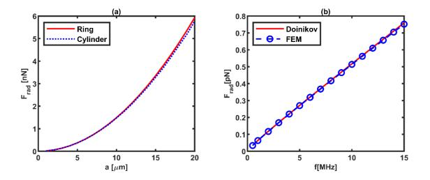
Fig 2.7. a) comparison of our numerical model for a ring and cylinder in water b) ARF versus frequency for a sphere in water compared with analytical results considering viscosity effects.
