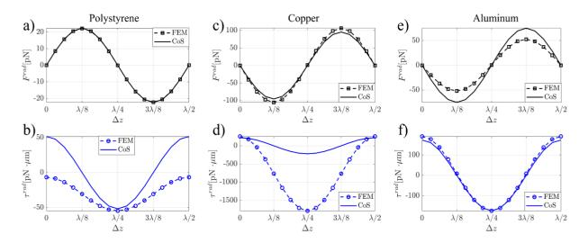
Fig 4.2. Comparison of the radiation forces ((a), (c) and (e)) and torques ((b), (d) and (f)) obtained from the FEM model and with the CoS method. (a) and (b) the results for polystyrene ring, (c) and (d) the results for copper ring and (e) and (f) the results for aluminum ring.
