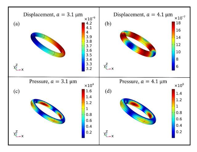
Fig 3.11. The displacement ((a)-(b)) and the pressure ((c)-(d)) distributions on non-resonating ((a) and (c)) and resonating ((b) and (d)) rings.
