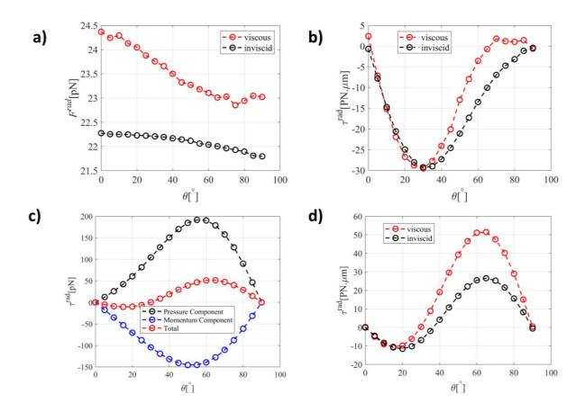
Fig 3.6. (a,b) comparison of Acoustic radiation forces and torques of inviscid and viscous fluids for  $\Delta z = \frac{\lambda}{8}$ , (c) Acoustic radiation torques and contribution of pressure and velocity for a polystyrene ring in viscous fluid for  $\Delta z = 0$ , (d) Comparison of acoustic radiation torque of inviscid and viscous fluid for  $\Delta z = 0$ .
