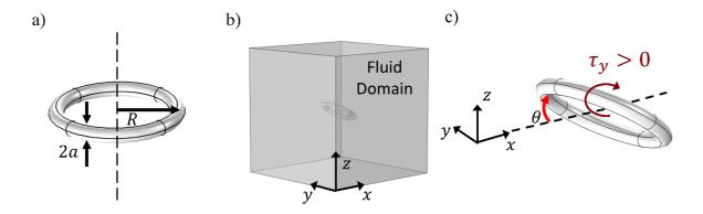
Fig 2.1. (a) Geometric parameters of the ring. (b) Ring is positioned inside a fluidic domain with radiation conditions at the boundaries in the simulation domain. (c) Ring rotation angle depiction,  $\theta$ .
