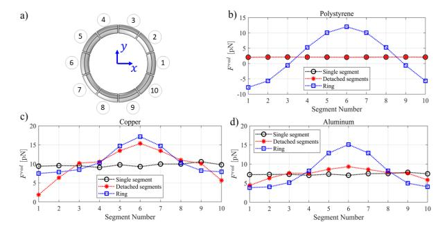
Fig 4.3. (a) The depiction of the ring decomposed into segments; local acoustic radiation forces (ARF) on each segment of polystyrene (b), copper (c) and aluminum (d) rings. ARF on each individual segment placed in the acoustic field without others is shown with black circles; forces on the detached segments forming a ring (see the picture in (a)) is shown with red stars; and the forces on the complete ring composed of segments in contact are shown with blue squares.
