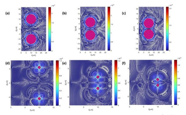
Fig 4.8. Streaming patterns and second-order velocity field are shown for polystyrene rings at f = 500 KHzand  $R = 10 \mu m$  with various inter-distances,  $d = 10,3,1 \mu m$  respectively (a-c) for  $a_1 = a_2 = 5 \mu m$ , (a-c) for  $a_1 = a_2 = 0.5 \mu m$ .
