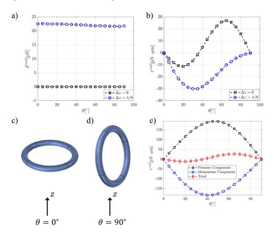
Fig 3.4. The change of (a)  $F^{rad}$  and (b)  $\tau^{rad}$  with respect to  $\theta$ . (c) shows the ring's orientation when  $\theta = 0^{\circ}$  and (d) shows the orientation when  $\theta = 90^{\circ}$ . The standing field is applied in the z- direction. (e) shows the pressure and momentum flux-driven component of the radiation torque on a polystyrene ring when  $\Delta z = 0$ .
