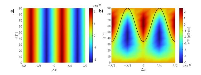
Fig 3.5. The change of (a)  $F^{rad}$  and (b)  $\tau^{rad}$  with respect to  $\theta - \Delta z$ . The standing field is applied in the z-direction on a polystyrene ring in an inviscid fluid when  $\theta$  varies between 0° and 90°.
