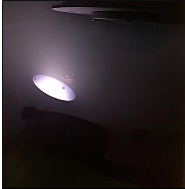
Figure 17. DC Sputtering of niobium target in AJA at 100 W DC power
