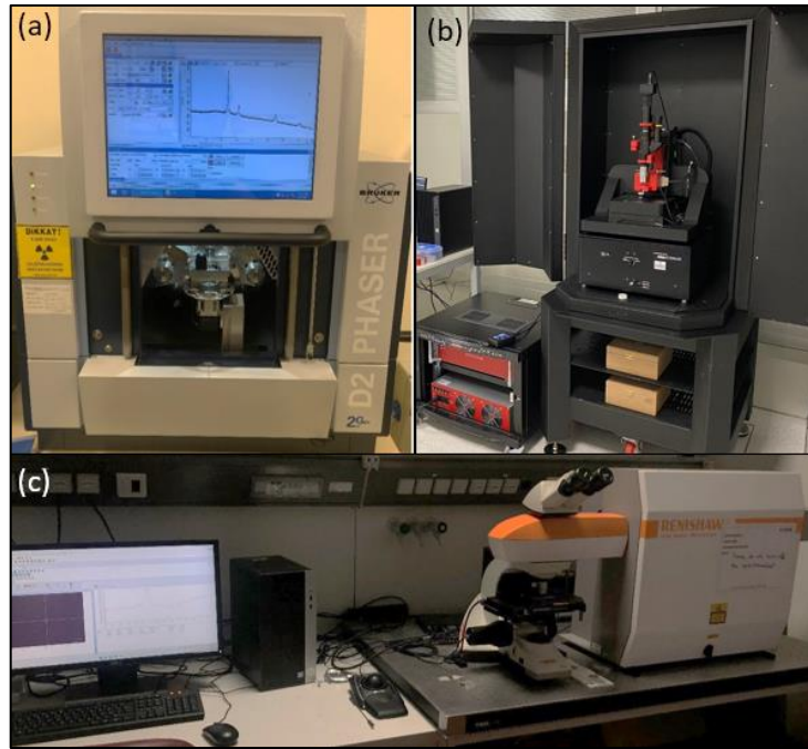
Figure 25. (a) Bruker D2 Phaser XRD System, (b) NanoMagnetic hp-AFM high performance atomic force microscope, (c) Renishaw Raman spectrometer
