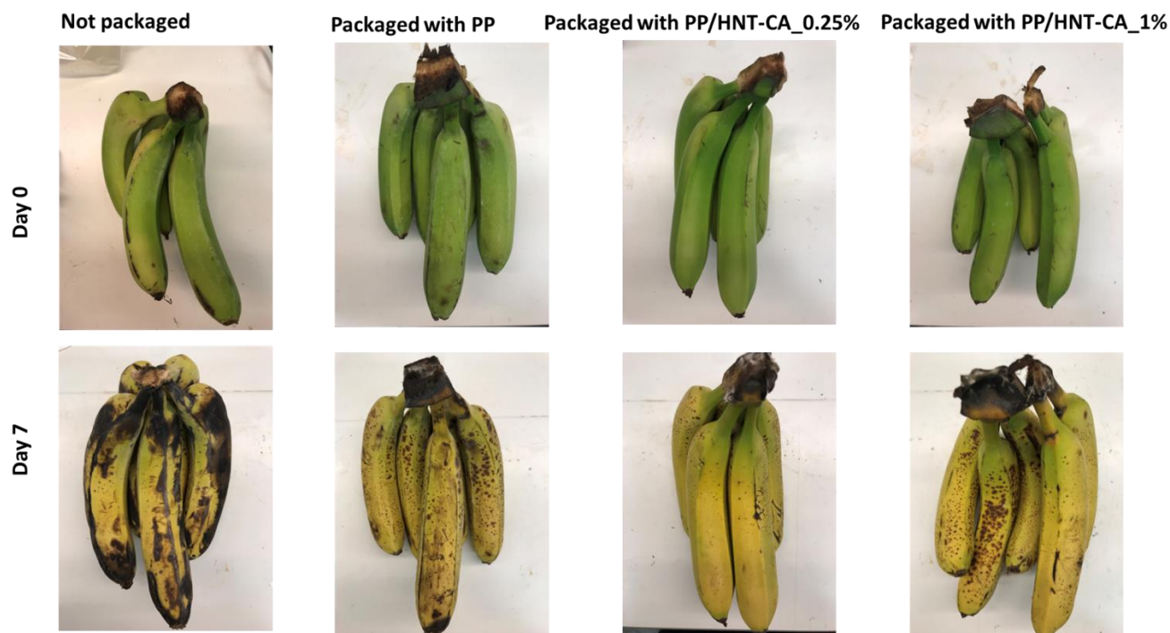
Figure 6. Photographs of not-packaged bananas, bananas packaged with PP, PP/HNT-CA_0.25%, and PP/HNT-CA_1% at day 0 and day 7.
