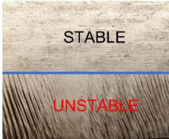
Figure 1.2. Surface finish with and without chatter
