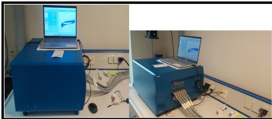
Figure 8: Biologic VMP 300 multipotentiostat used for Electrochemical analysis located at FENS lab (2110) at Sabanci University.
