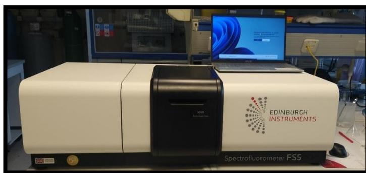
Figure 7: Spectrofluorometer FS5 for PL analysis located at FENS lab (2110) at Sabanci University.
