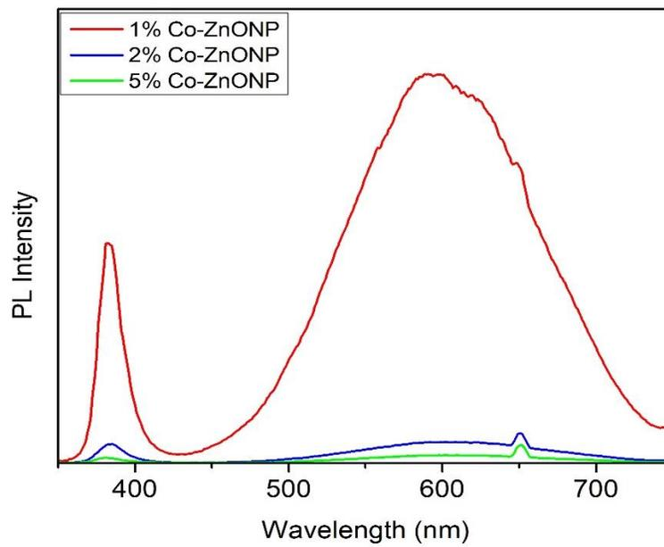
Figure 27: PL Spectra of Co-doped ZnONPs at 1, 2, and 5 % doping concentration.
