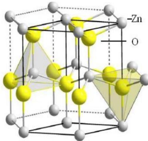
Figure 3: Crystal Structure of ZnO [23].
