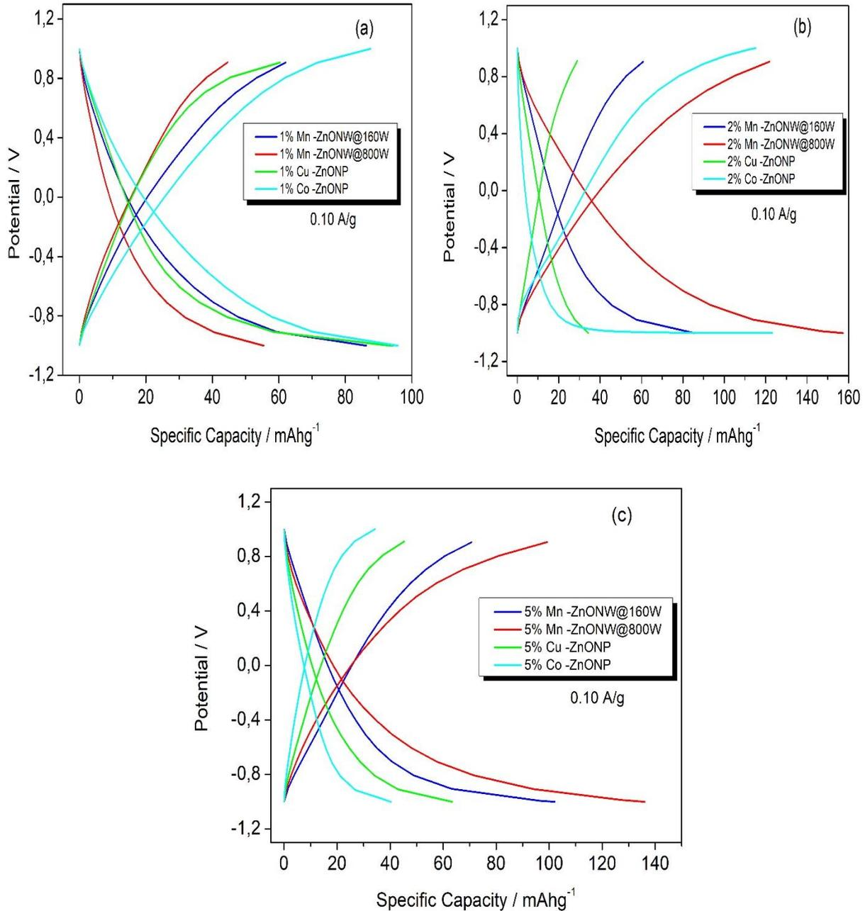
Figure 35: Galvanostatic charge-discharge curves of supercapacitor designs at 0.10 A/g current density: a) 1% doped samples, b) 2% doped samples, and c) 5% doped samples.
