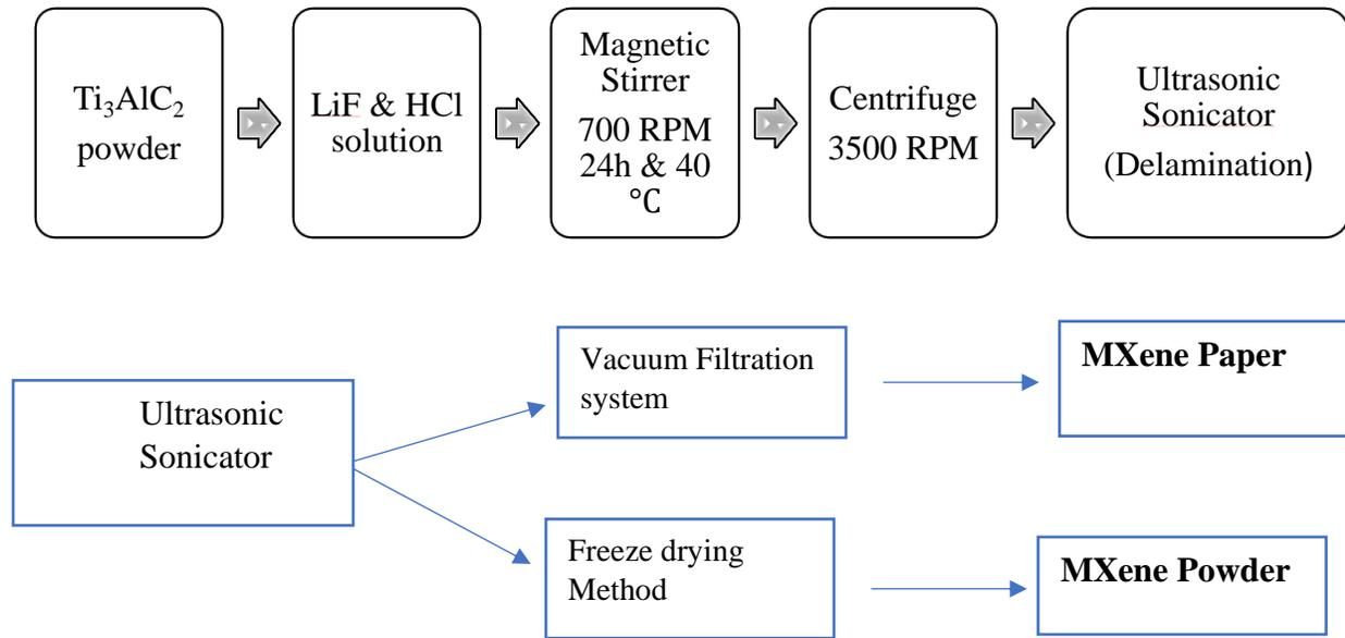
Figure 5: Flow chart of MXene synthesis
