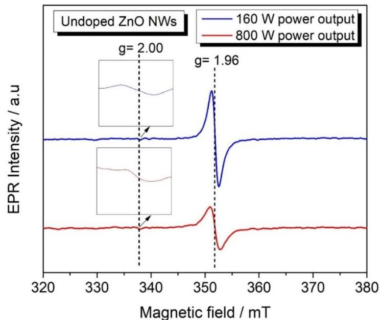
Figure 19: EPR spectra of Undoped ZnONW at 160W and 800W.
