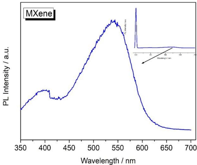
Figure 28: PL emission spectra of MXene excited at 300 nm.
