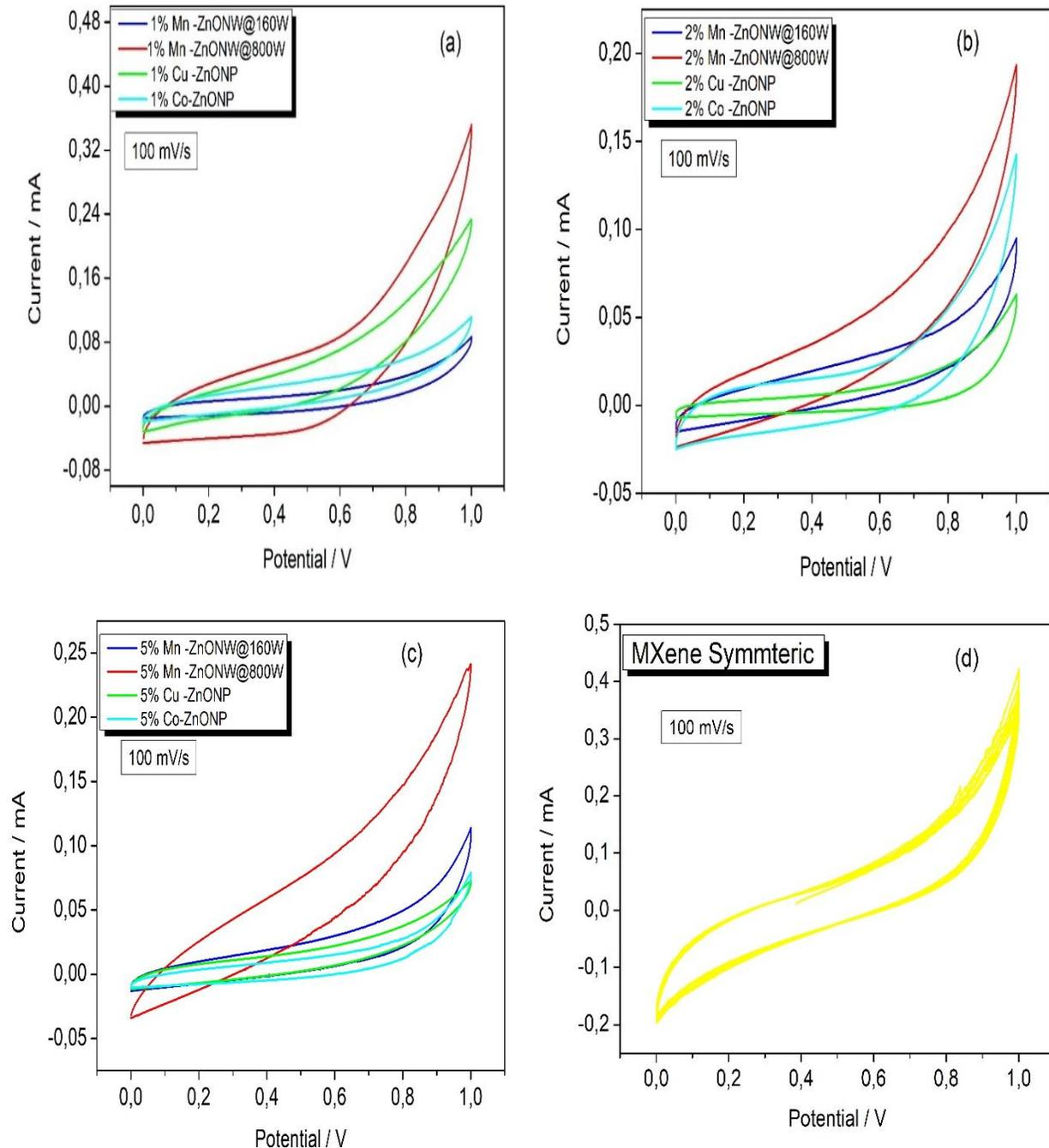
Figure 30: Cyclic Voltammetry scans supercapacitor designs: a) 1% doped samples, b) 2% doped samples, c) 5% doped samples, and d) MXene symmetric.
