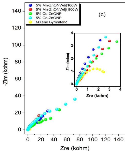
Figure 32: Electrochemical impedance spectra (Nyquist plot) of supercapacitor designs: a) 1% doped samples b) 2% doped samples and c) 5% doped samples.
