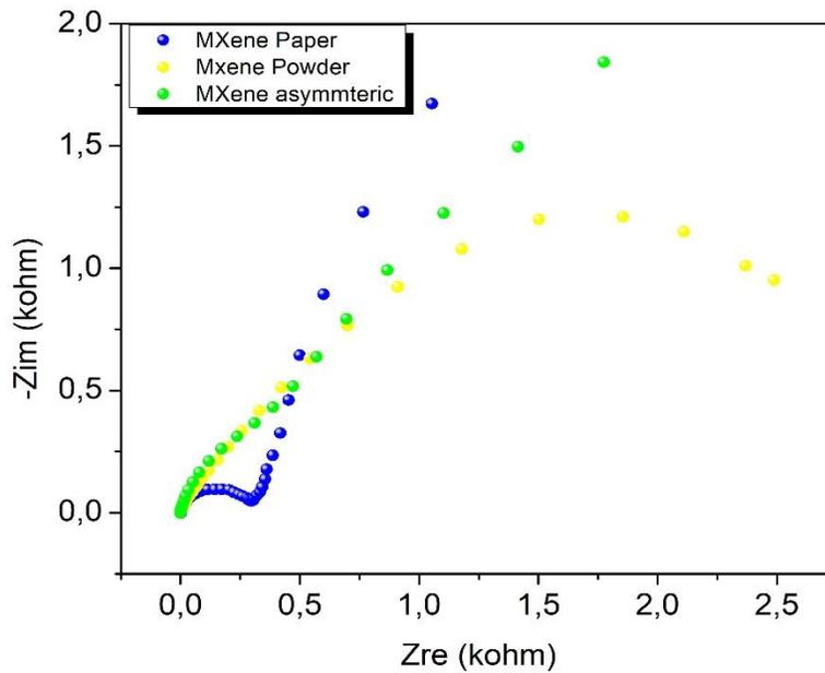
Figure 34: Nyquist plot for MXene-based supercapacitor.
