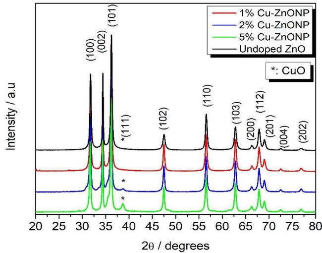
Figure 10: XRD pattern of Cu-doped ZnONP at 1, 2, and 5 % doping concentration.
