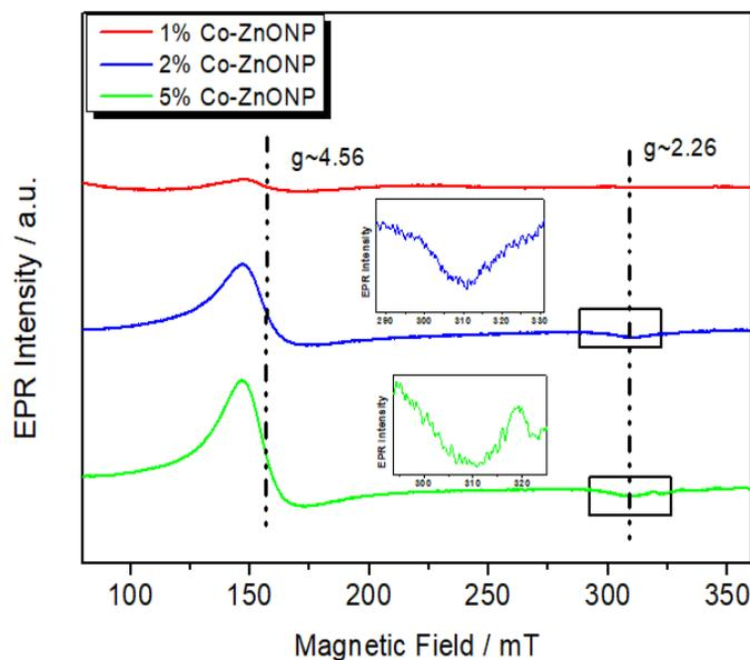
Figure 22: EPR Spectra of Co-doped ZnONP at 1, 2, and 5 % doping concentration.
