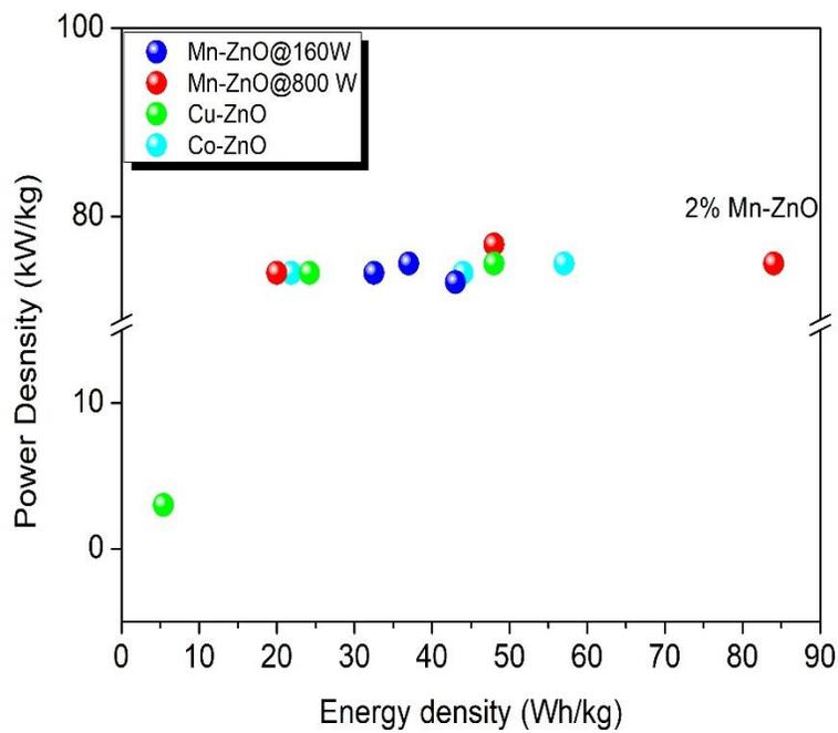
Figure 38: Ragone plot for metal oxide-based supercapacitor designs
