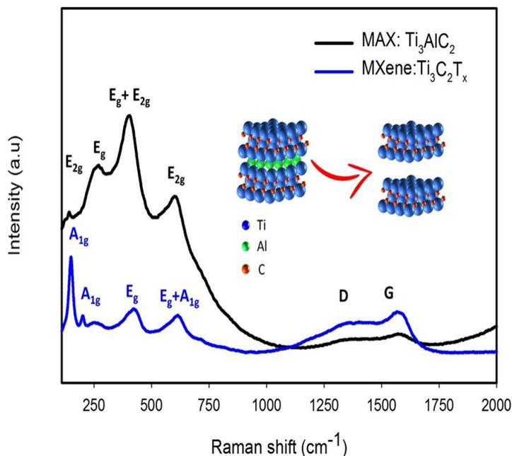
Figure 17: Raman spectra of MAX phase ( $\text{Ti}_3\text{AlC}_2$ ) and MXene ( $\text{Ti}_3\text{C}_2\text{T}_x$ ).
