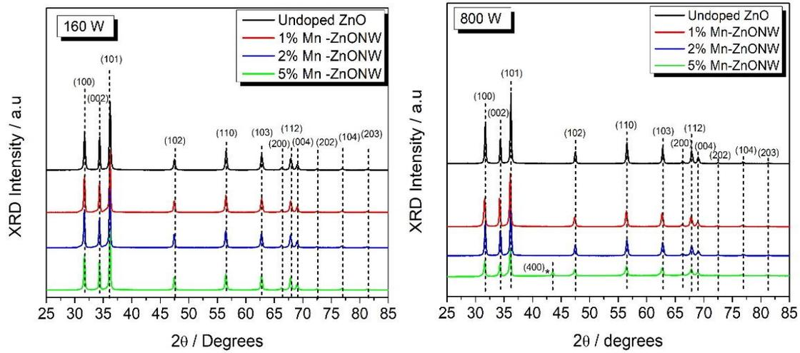
Figure 9: XRD pattern of Mn-doped ZnO NW at 1, 2, and 5 % doping concentration synthesized at 160 W (left) and 800 W (Right).
