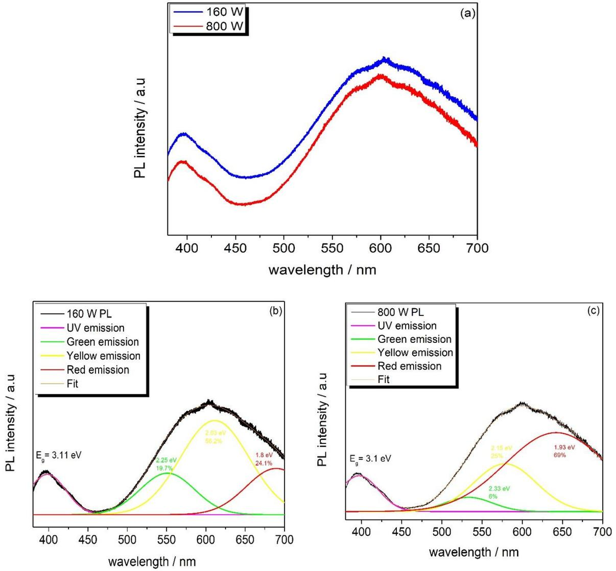
Figure 24: (a) PL spectra of undoped ZnONW at 160W and 800W (b) Deconvolution of 160 W PL (c) Deconvolution of 800 W PL.
