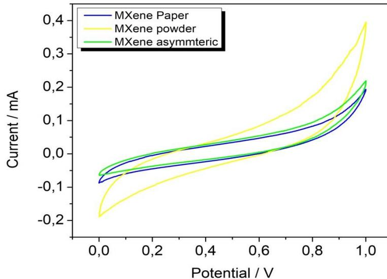
Figure 31: Cyclic Voltammetry scans supercapacitor designs for MXene-based electrode.
