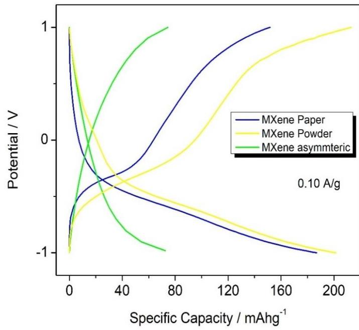
Figure 36: Galvanostatic charge-discharge curves of MXene-based supercapacitor designs.
