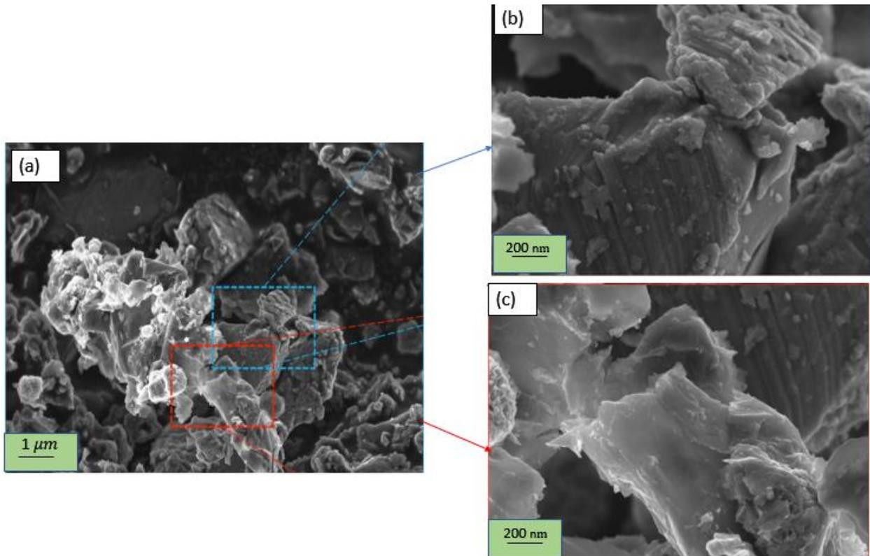
Figure 14: SEM images of Ti<sub>3</sub>AlC<sub>2</sub> (MAX Phase).
