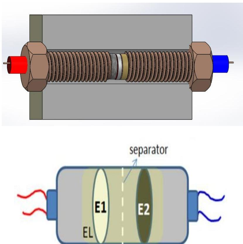
Figure 29: Supercapacitor design and schematic representation.
