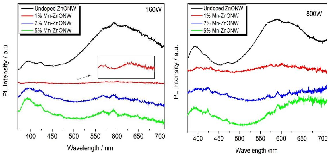
Figure 25: PL spectra of Mn-doped ZnONWs at 1, 2, and 5 % doping concentration synthesized at 160 W(left) and 800 W (Right).
