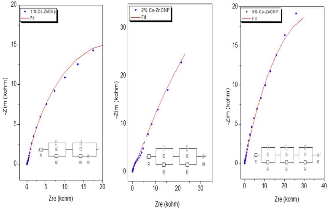
Figure 33: Equivalent circuit used to fit the Nyquist plot experimental data.
