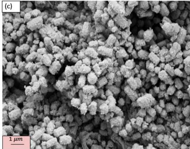
Figure 13: SEM images of (a) Mn-doped ZnO NW, (b) Cu-doped ZnO NP, and (c) Co-doped ZnO NP.
