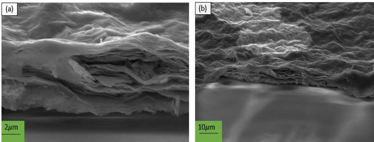
Figure 15: SEM images of  $Ti_3C_2T_x$  (MXene).
