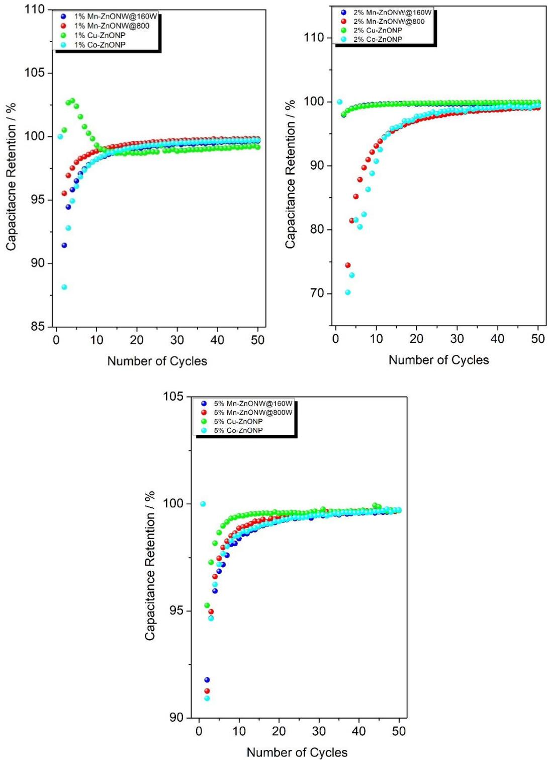
Figure 37: Capacitance retention of supercapacitor designs at a current density of 0.15 A/g
