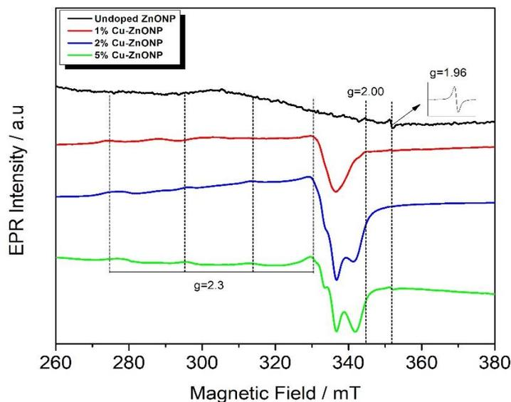
Figure 21: EPR Spectra of Cu-doped ZnONP at 1, 2, and 5 % doping concentration.
