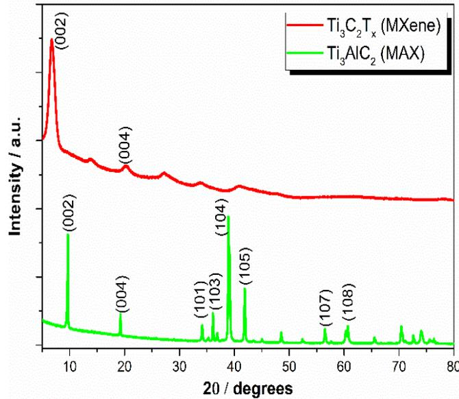
Figure 12: XRD pattern for  $Ti_3AlC_2$  (MAX) and  $Ti_3C_2T_x$  (MXene).
