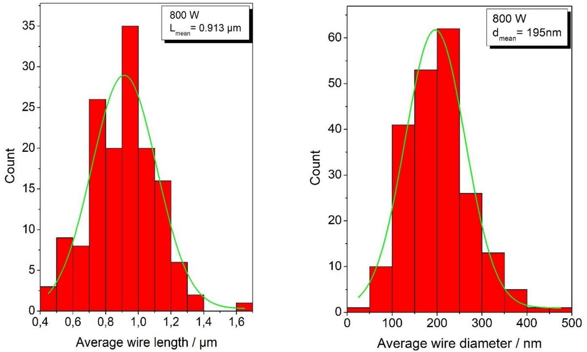
Figure 16: Aspect ratio histogram of undoped ZnO nanowires
