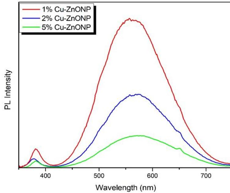
Figure 26: PL Spectra of Cu-doped ZnONPs at 1, 2, and 5 % doping concentration.
