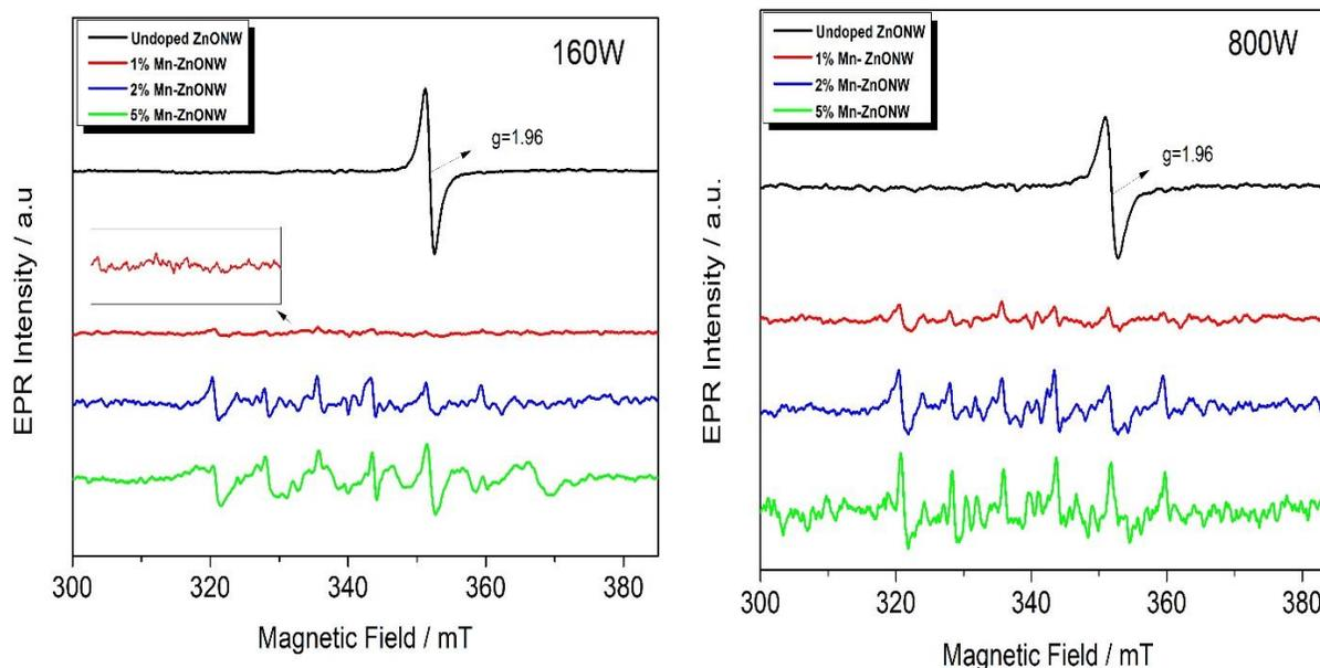
Figure 20: EPR spectra of Mn-doped ZnONW at 1, 2, and 5 % doping concentration synthesized at 160W(left) and 800W (Right).
