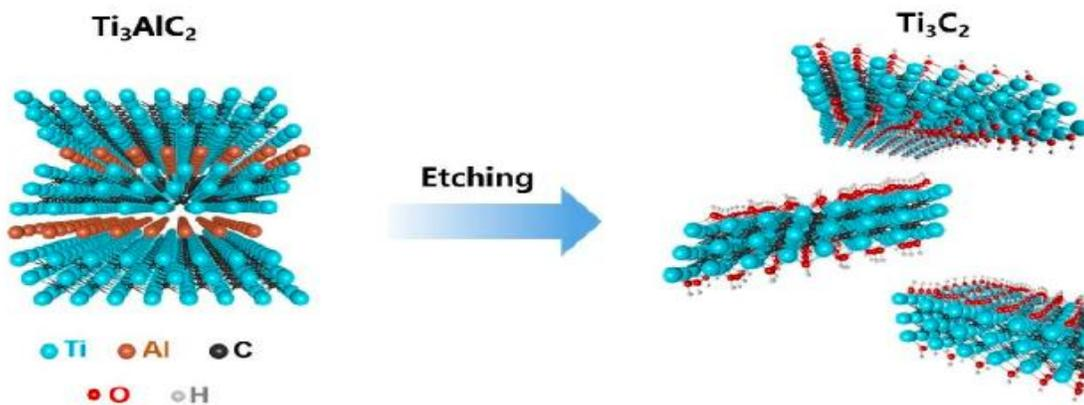
Figure 4: Selective etching of MAX phase to MXene [55]
