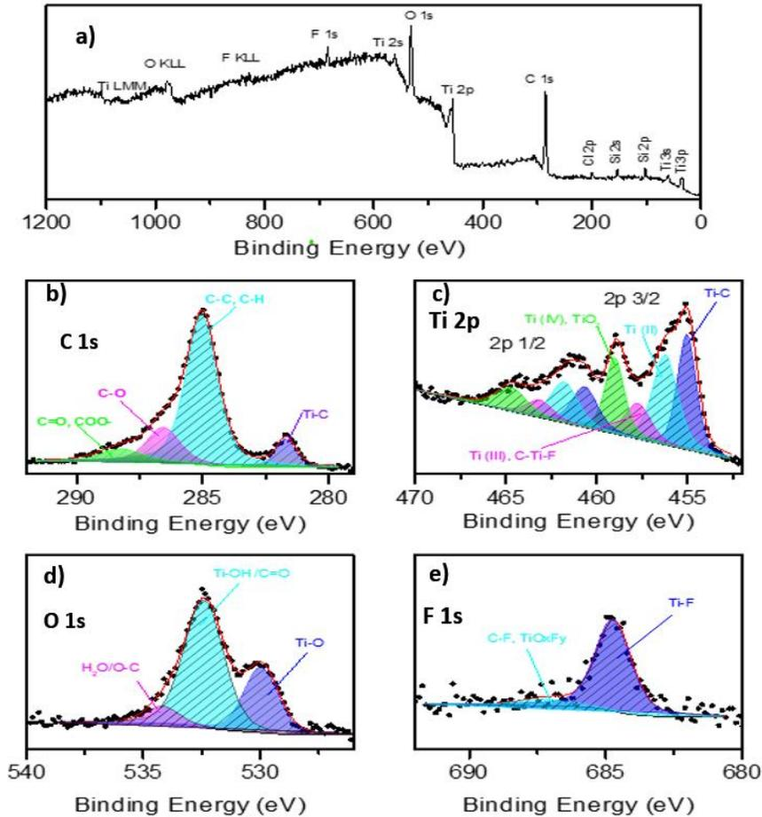
Figure 18: XPS spectra of MXene ( $\text{Ti}_3\text{C}_2\text{Tx}$ ) powder: (a) survey, (b–e) high resolution spectra of C 1s, Ti 2p, O 1s, and F 1s regions, respectively.
