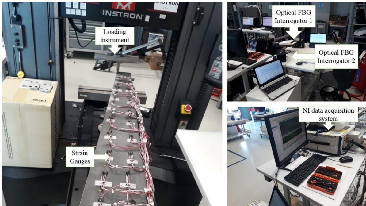
Fig. 3-12. Experimental deployment of the sensors on the laminate and strain-data collection systems.
