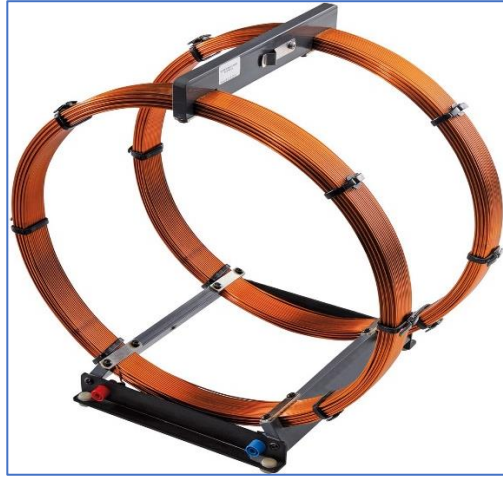
Figure 27. Helmholtz coils produce an external magnetic field.
