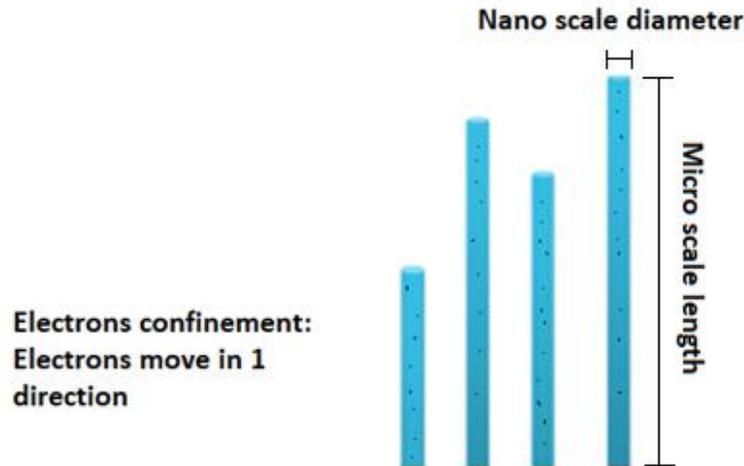
**Figure 7:** Electrons confinement and movement in 1 direction due to NWs morphology.
