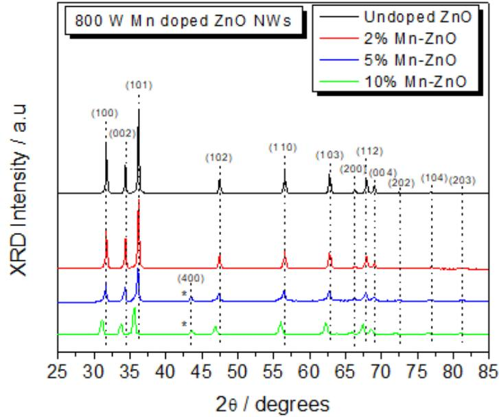
**Figure 12:** XRD plots for Mn-doped ZnO samples with varying Mn concentrations synthesized with 800 W microwave power.
