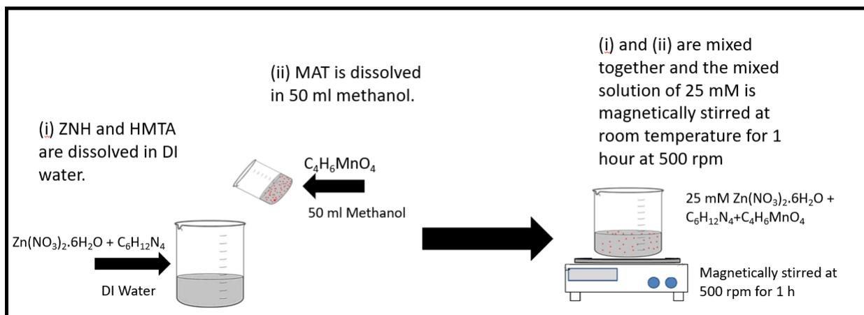
**Figure 9:** Schematic representation of the microwave-assisted hydrothermal synthesis of pure and Mn-doped ZnO NWs.
