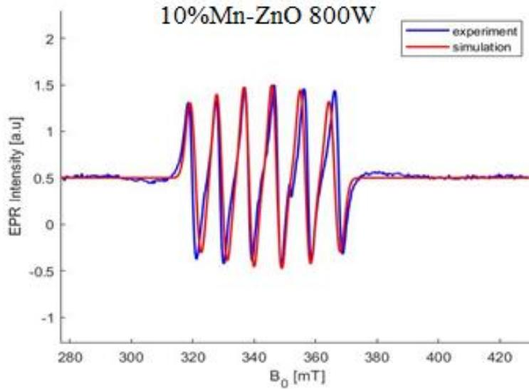
**Figure 25:** EPR data simulation of 10% Mn-ZnO NWs synthesized with 800 W microwave power.
