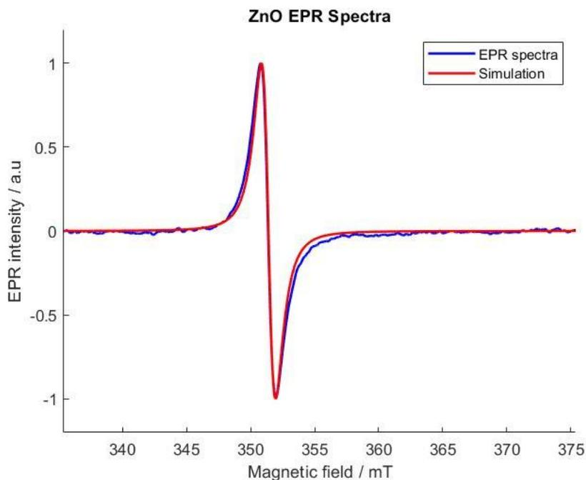
**Figure 20:** EPR data simulation of pure ZnO synthesized by the microwave-assisted hydrothermal method by using “pepper” function of Easyspin in Matlab.
