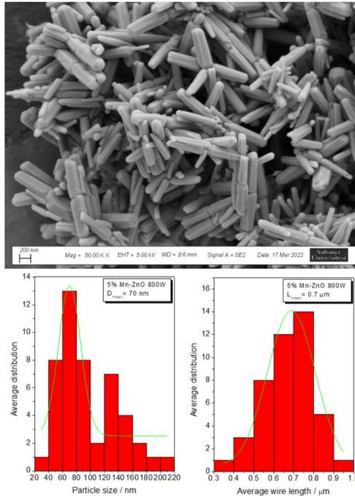
**Figure 16:** SEM image of 5%Mn-ZnO synthesized by microwave-assisted hydrothermal method, histograms of average wires diameter and length below the image.
