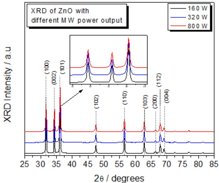
**Figure 10:** XRD plots of pure ZnO NWs produced with different microwave power outputs.
