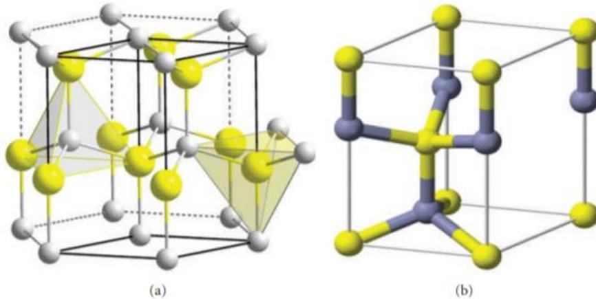
**Figure 5:** ZnO crystal structure (yellow Zn – grey O) (a) hexagonal wurtzite structure (b) hexagonal wurtzite unit cell (adopted from [9]).
