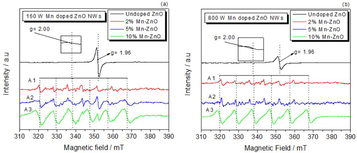
**Figure 24:** EPR spectra of pure and Mn-doped ZnO NWs synthesized with (a) 160 W microwave power and (b) 800 W microwave power.
