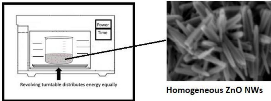
**Figure 8:** Homogenous growth of ZnO NWs by the microwave-assisted method.
