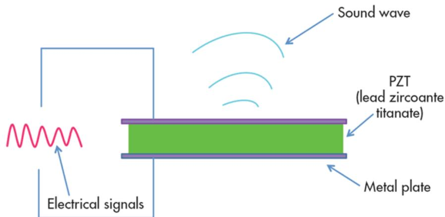
**Figure 3:** Working principle of reverse piezoelectric effect (adapted from: [11]).
