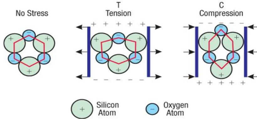
**Figure 4:** Piezoelectric effect in quartz crystal (adapted from: [11]).
