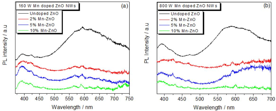
**Figure 29:** PL spectra of pure and Mn-doped ZnO samples synthesized with (a) 160 W and (b) 800 W microwave powers.
