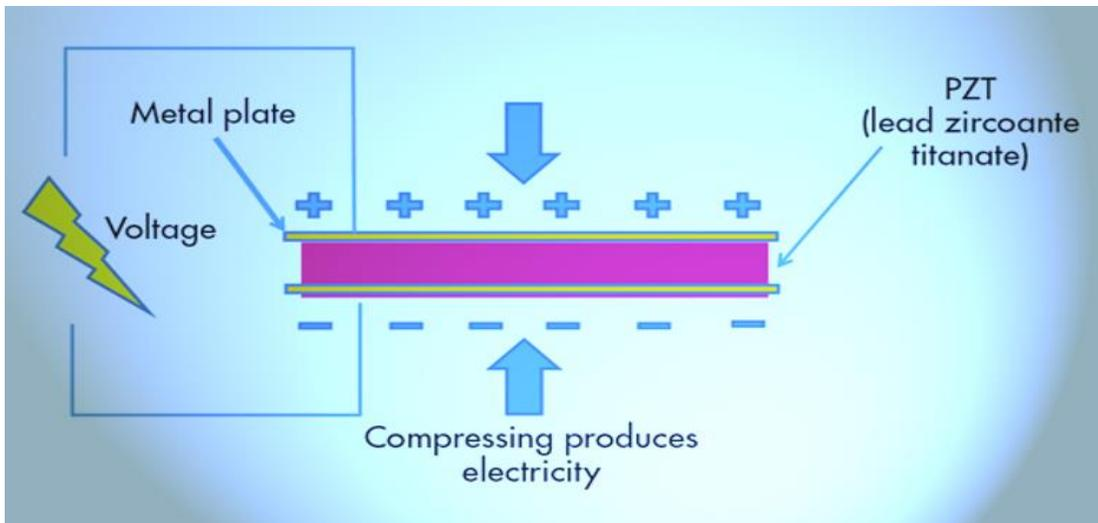
**Figure 2:** Working principle of direct piezoelectric effect (adapted from: [11]).
