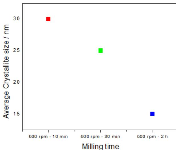
**Figure 14:** Effect of ball-milling time on average crystallite size.
