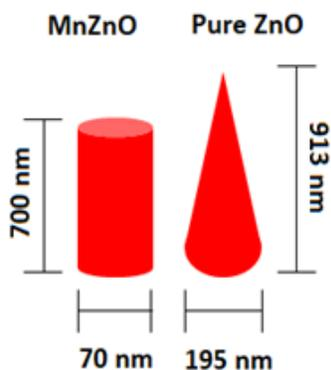
**Figure 17:** Comparison between Pure and Mn-doped ZnO nanowires.
