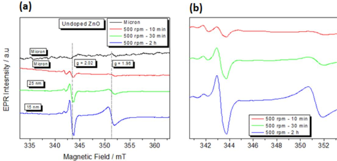
**Figure 21:** (a) EPR spectra of ball-milled pure ZnO samples as a function of ball-milling time
