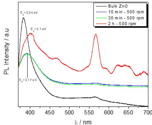
**Figure 28:** PL spectra of ball-milled ZnO samples as a function of milling time.
