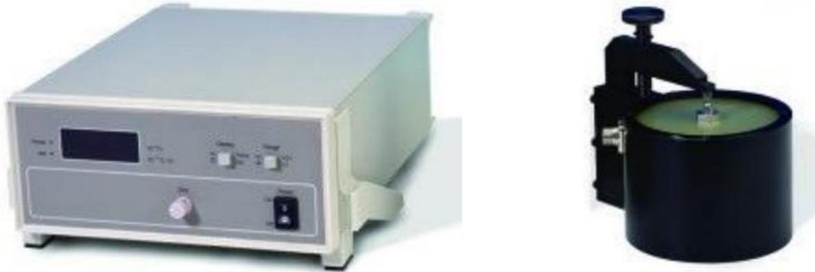
**Figure 31:** Main components of D33PZO1 measurement device.
