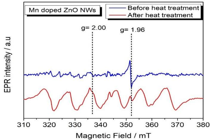
**Figure 26:** EPR spectra of 10%Mn-ZnO sample before and after heat treatment.
