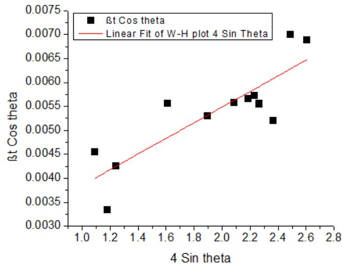
**Figure 11:** W-H Plots linear fitted line.
