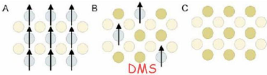
**Figure 6:** (A) Magnetic semiconductor (B) DMS (C) Nonmagnetic semiconductor (adapted from: [20]).
