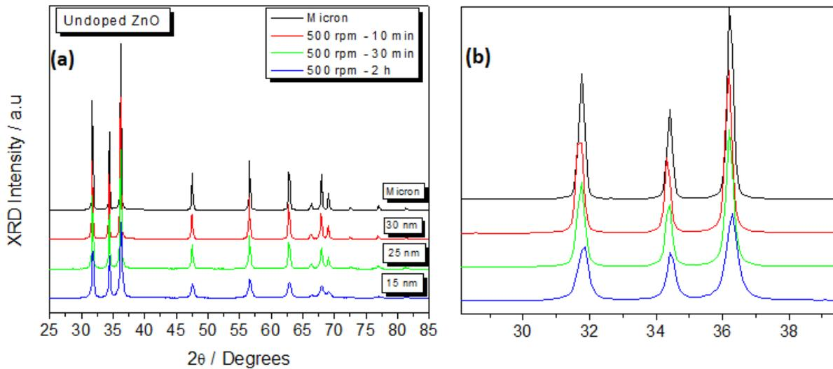
**Figure 13:** (a) XRD plot for pure ZnO samples with varying milling times (b) peak broadening of the main 3 peaks.
