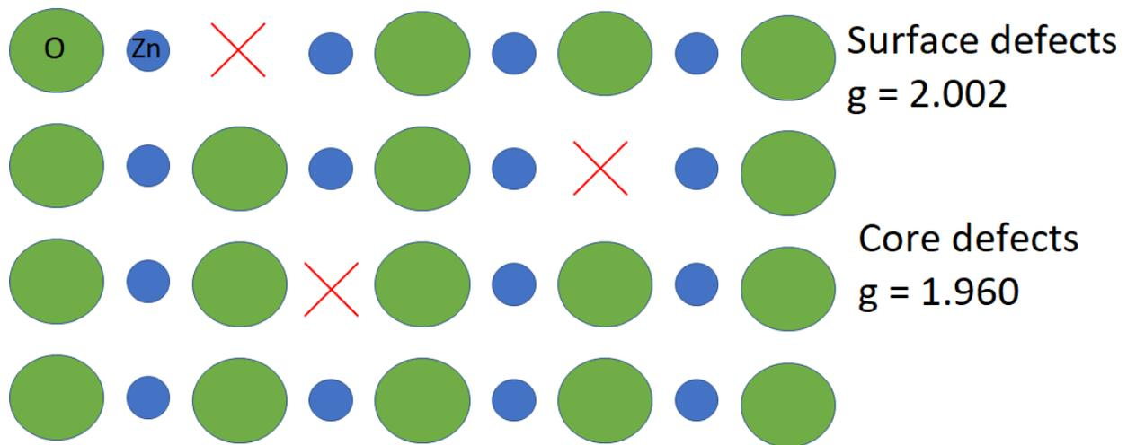
**Figure 19:** Surface and core defects of ZnO structure due to shielding of core signal.
