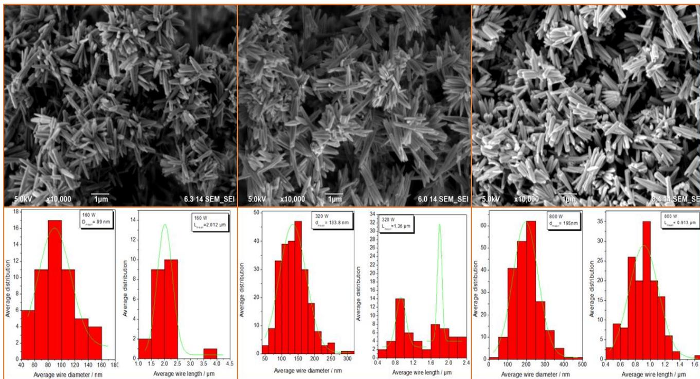
**Figure 15:** SEM images and histograms of average wire diameter and length for ZnO samples with microwave power outputs of 160 W, 380 W, and 800 W from left to right.
