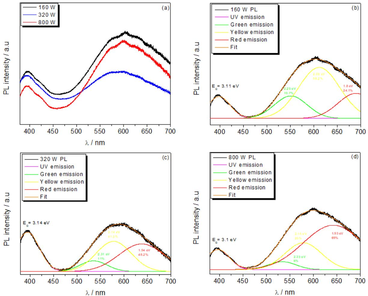
**Figure 27:** (a) PL spectra of pure ZnO samples synthesized via the microwave-assisted hydrothermal method with varying microwave powers. (b) Deconvolution of 160 W PL. (c) Deconvolution of 320 W PL. (d) Deconvolution of 800 W PL.
