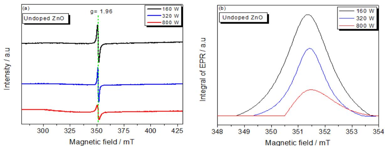
**Figure 18:** (a) EPR spectra of pure ZnO samples synthesized with varying microwave power outputs (b) Integrated EPR spectra.
