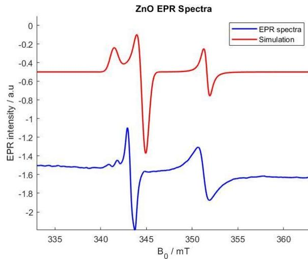
**Figure 23:** EPR data simulation of 2 hours ball-milled pure ZnO sample by using the “pepper” function.
