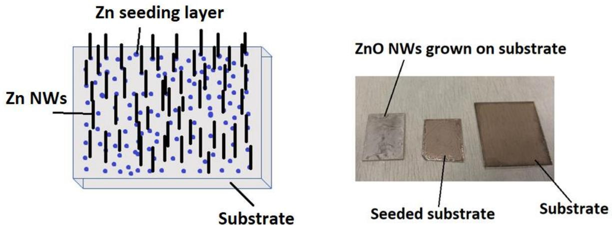
**Figure 30:** Schematic of the effect of the seeding layer, and ZnO NWs growth on a substrate in the lab.
