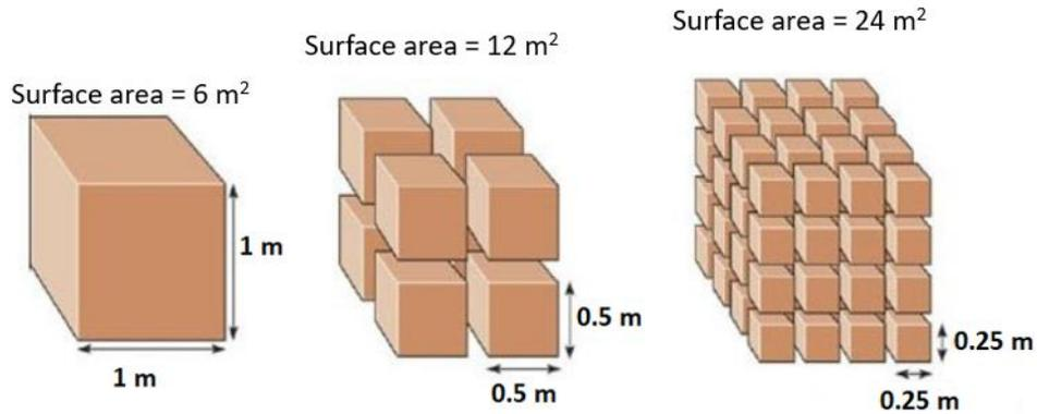
**Figure 22:** Surface area to volume ratio as a function of decreasing crystallite size (adapted from [51]).
