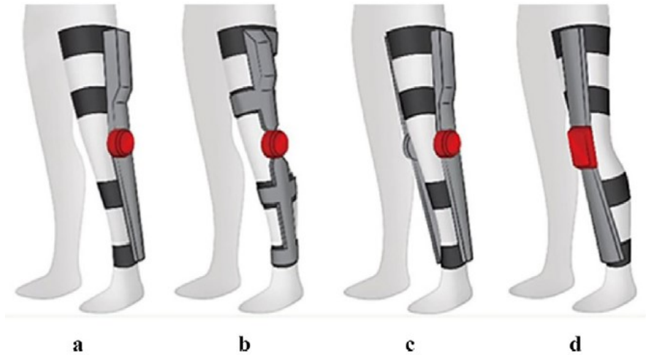
Figure 2.4 a) lateral-support layout; b) improved lateral-support layout; c) two-side-support layout; d) anterior/posterior-support layout [3]
