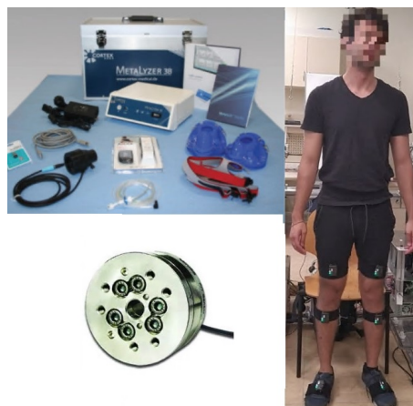
Figure 5.1 Cortex Metalyzer 3B spirometry device, I-sens inertial motion capture system, ATI force sensor
