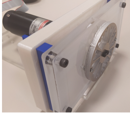
Figure 3.14 Experimental verification setup for compliant torsional stiffness mechanism
