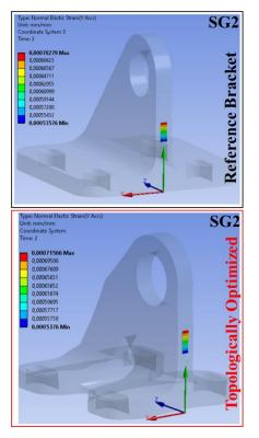
**Fig 6.** FEA analyses on the bracket showing elastic strains of the regions where the maximum strain is obtained based on DIC test.
