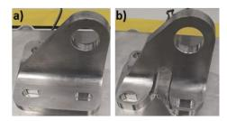
Fig 5. Captured images of a) reference b) topologically optimized bracket.
