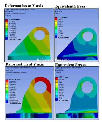
**Fig 7.** FEA analyses demonstrating bracket's deformation, and equivalent stress distribution.
