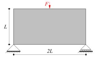
Fig 3. Design domain of the simply supported beam.
