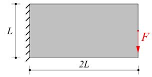
Fig 5. Design domain of the cantilever beam.
