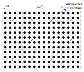
**Fig 2.** Schematic of microcrack in a design domain, black circles represent the particles in PD, the grid of 4 by 4 is located between dashed lines; red lines are microcracks with the size of  $L_{crack}$  and orientation of  $\theta$ .
