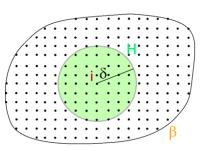
Fig 1. Horizon-Family of the material point *i* for PD model.
