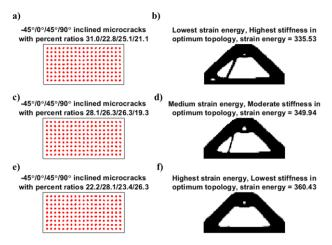
**Fig 7.** Simply supported beam with sets of microcracks  $(L_{crack} = dx)$ , a) microcracks orientation for achieving minimum strain energy, b) optimum topology for minimum strain energy, c) microcracks orientation for achieving medium strain energy, d) optimum topology for medium strain energy, e) microcracks orientation for achieving maximum strain energy, f) optimum topology for maximum strain energy.
