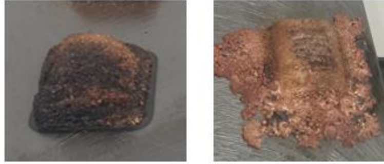
Figure 12 Failed CuSn10 trials due to overheat and overdeposition
