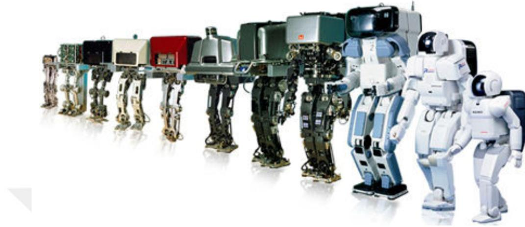
Figure 2.3 HONDA's humanoid robot family includes the following models: E0-6, P1-3, and ASIMO (Yampolskiy & Gavrilova, 2012)
