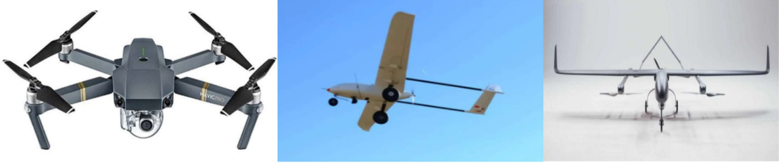
Figure 2.1: Left: Rotary Wing DJI Quadcopter. Middle: Fixed Wing AA Albatross. Right: PD1 UKR Hybrid
