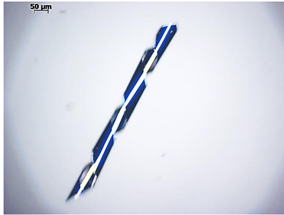
Fig. 3.14. The new swimmer with 150 nm sandwich nickel
