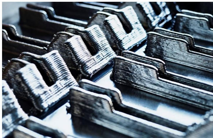
Figure 2-4 First DED AM structural airplane component - Boeing 787 Dreamliner.
