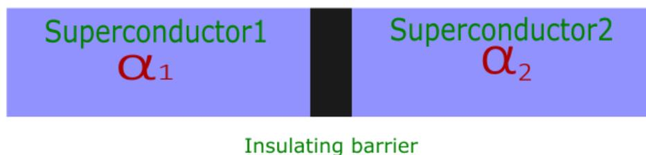
Figure 2.1. Schematic of a Josephson junction. Superconductor 1 with phase  $\alpha_1$  and superconductor 2 with phase  $\alpha_2$  which are separated by a thin insulating barrier.
