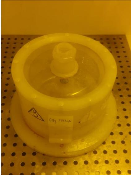
Figure 3.1 Photograph of spin coater at SUNUM
