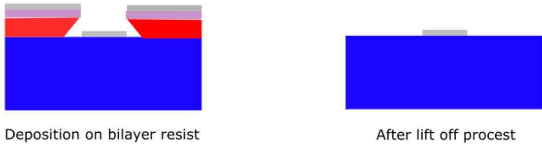
*Figure 3.7 Schematic of lift off process*
