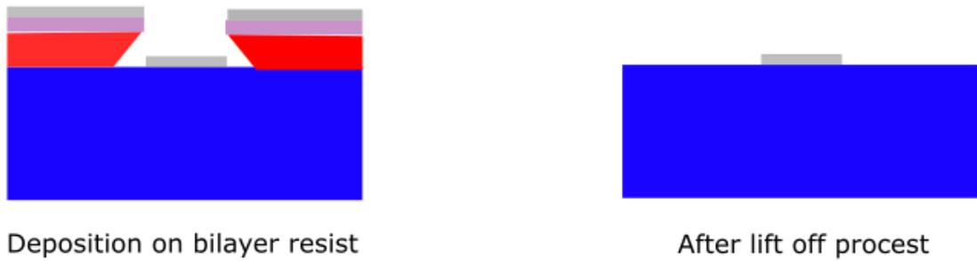
*Figure 3.7 Schematic of lift off process*
