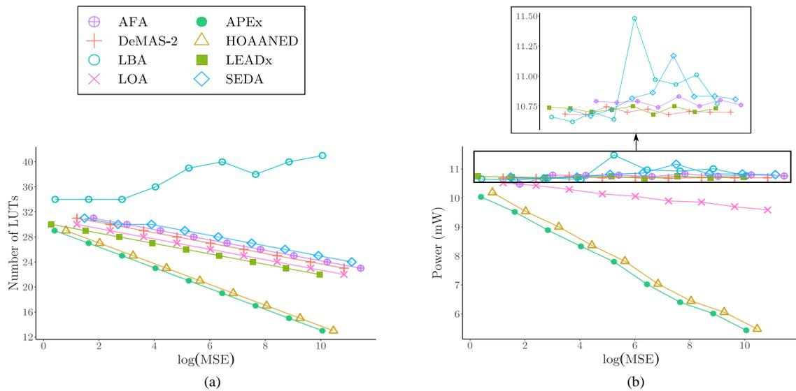
**Figure 5.9** Comparison of 32-bit approximate adders with 4-bit to 20-bit approximation (left to right). (a) LUTs vs MSE. (b) Power vs MSE.
