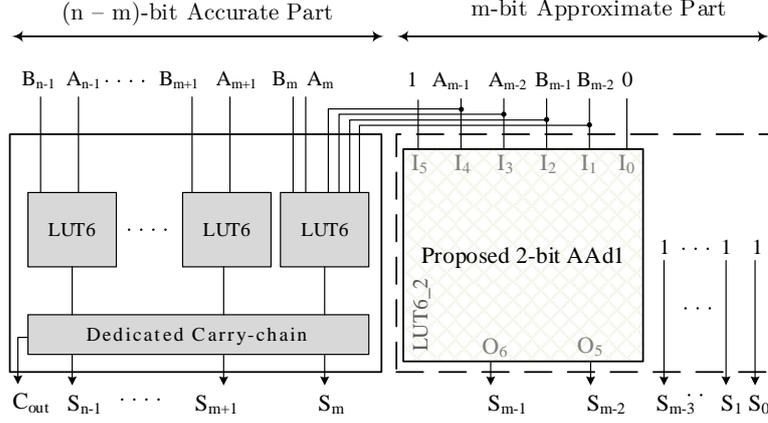
**Figure 5.6** Proposed n-bit area and power efficient approximate adder (APEX).
