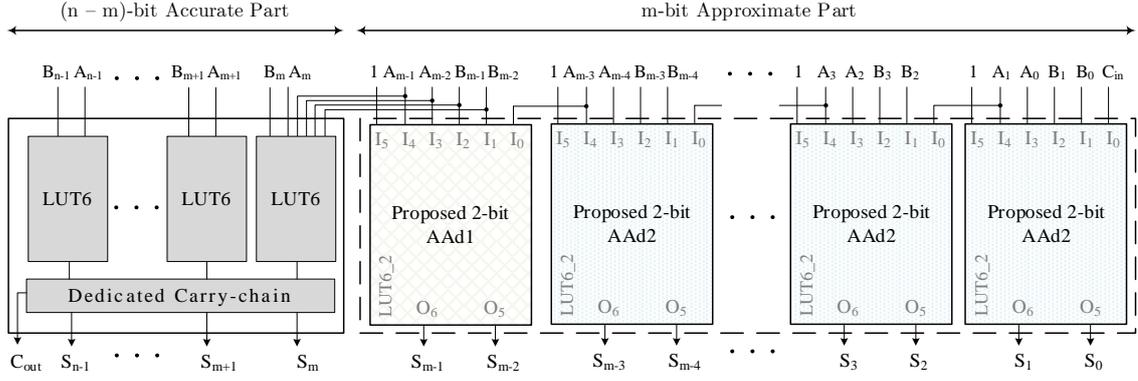
**Figure 5.4** Proposed  $n$ -bit low error and area efficient approximate adder (LEADx).
