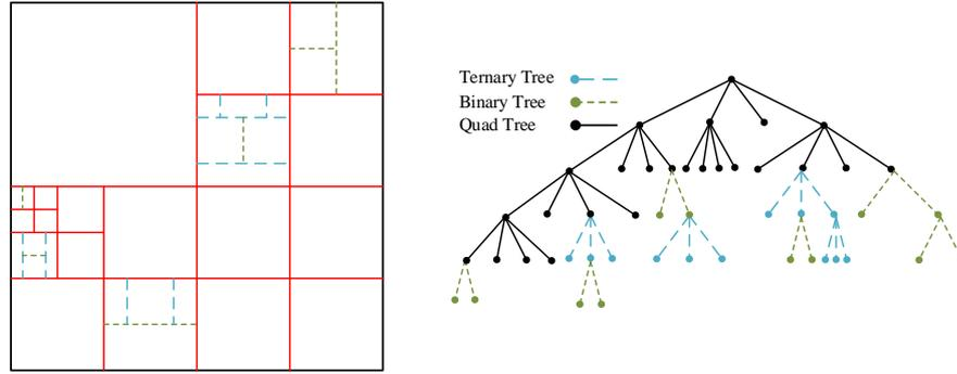
**Figure 3.2** An example of QTMT partitioning of 128x128 CTU and its decision tree.
