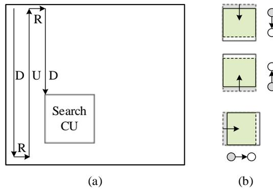
**Figure 3.7** (a) Vertical snake scan order (b) Data re-use in downward, upward, and right directions.
