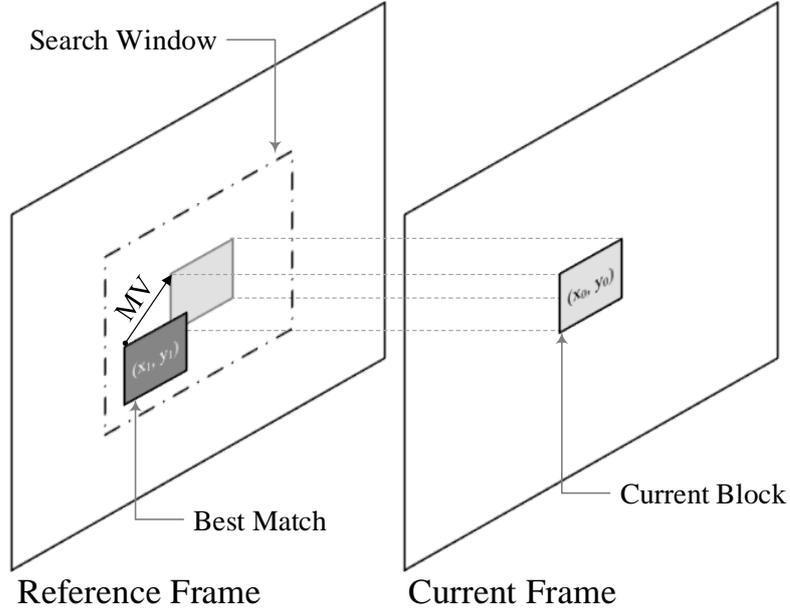
**Figure 1.7** The motion estimation process
