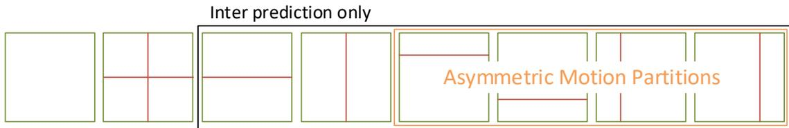
**Figure 1.6** Partitioning of a CU into a PU in HEVC
