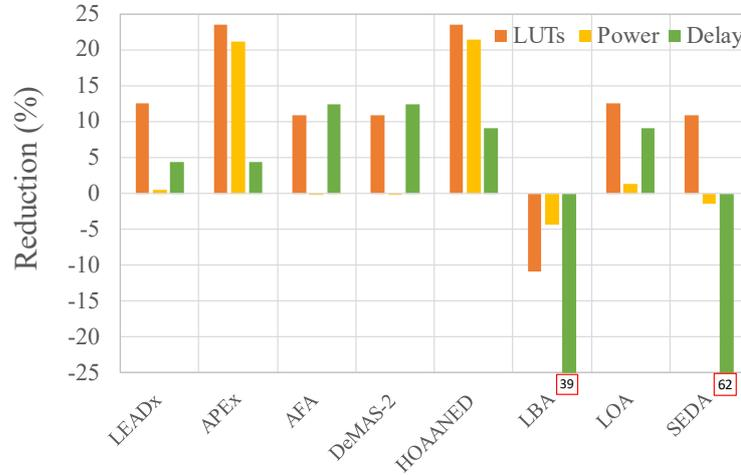
**Figure 5.10** Area, Power, and Delay reduction achieved with 16-bit approximation in 64-bit approximate adders compared to 64-bit accurate adder.
