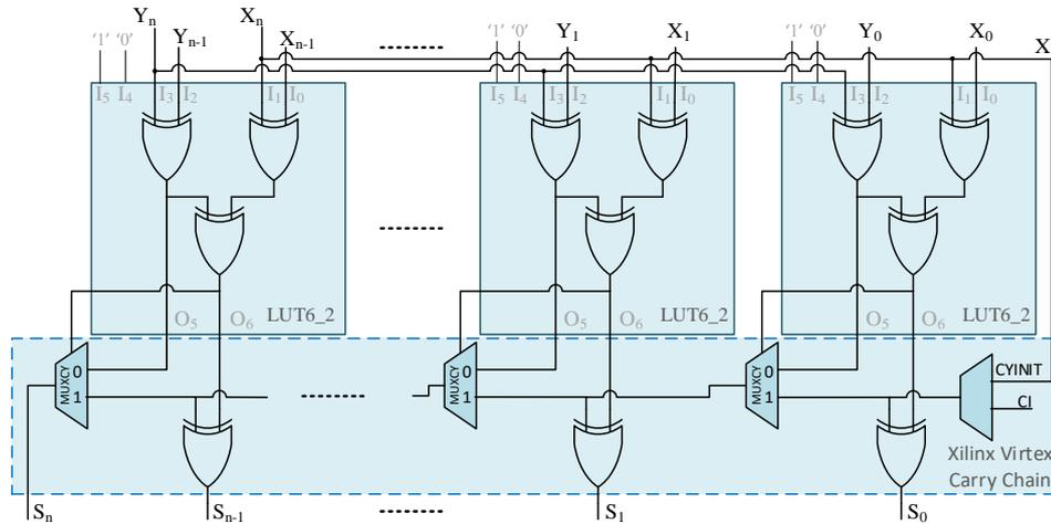
**Figure 4.5** Implementation of the proposed n-bit adder/subtractor including complement operations
