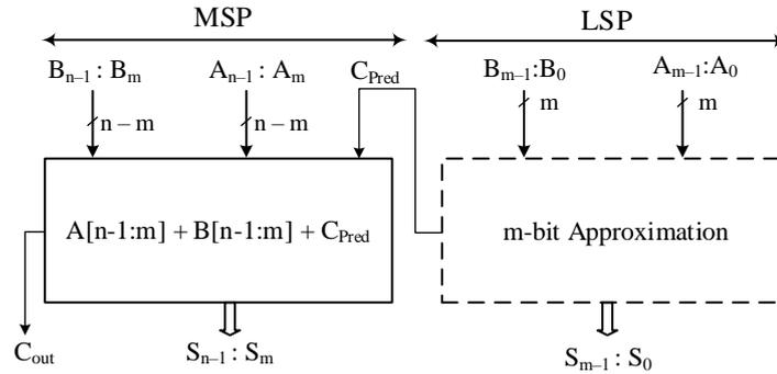
**Figure 5.1** Architecture of approximate full-adder based n-bit approximate adders
