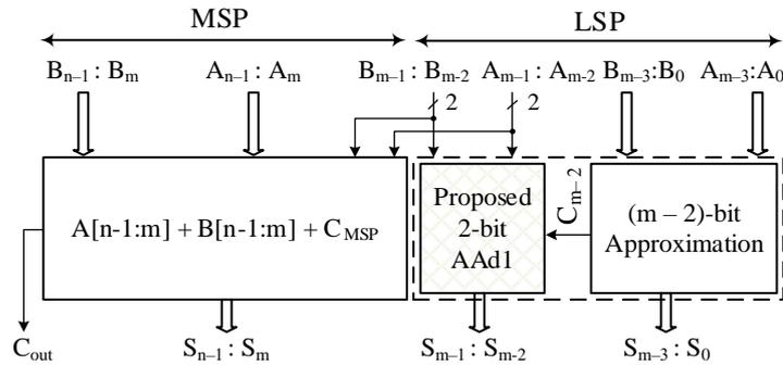
**Figure 5.3** Architecture of proposed approximate adders for FPGAs.
