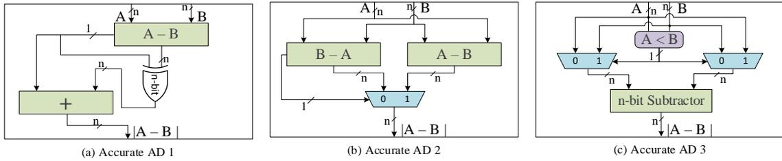
**Figure 4.2** Accurate absolute difference hardware
