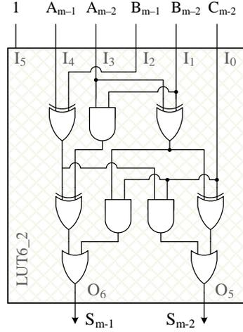
**Figure 5.2** Proposed 2-bit approximate adder (AAd1) used in MSBs of LSP.
