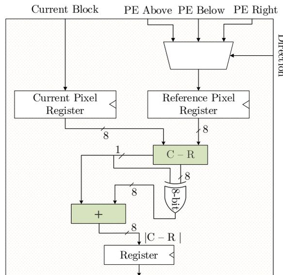
**Figure 3.6** Processing Element (PE)
