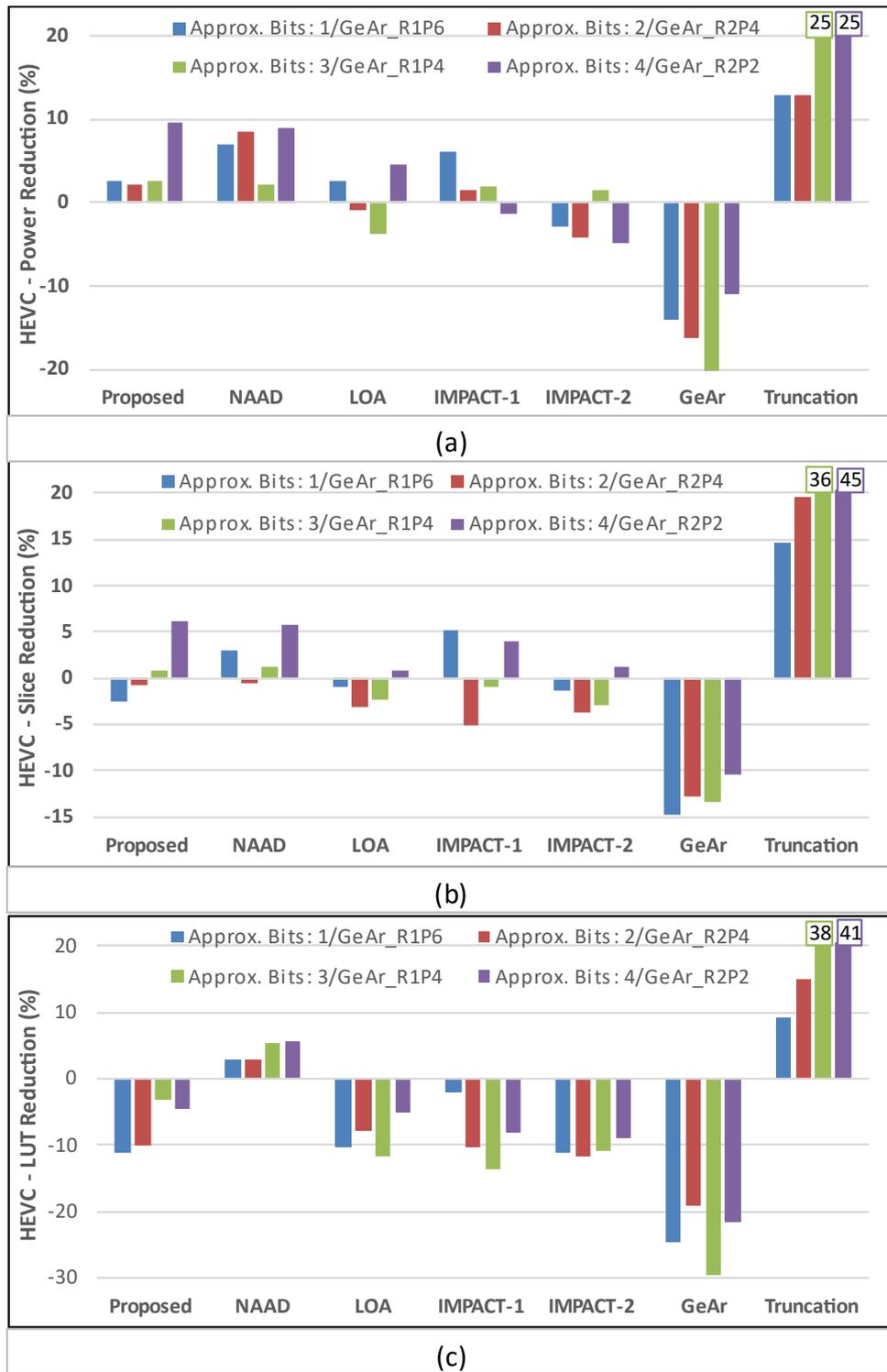
Figure 2.10 (a) Power Reduction (%) (b) Slice Reduction (%) (c) LUT Reduction (%)
