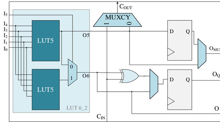
**Figure 4.3** Simplified architecture of a slice in Xilinx Virtex 5/6/7 FPGAs
