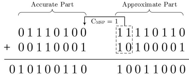
**Figure 5.5** Example of 16-bit LEADx with 8-bit approximation.
