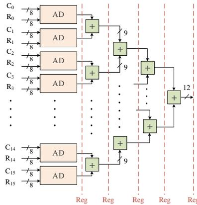
**Figure 3.8**  $4 \times 4$  SAD calculation.
