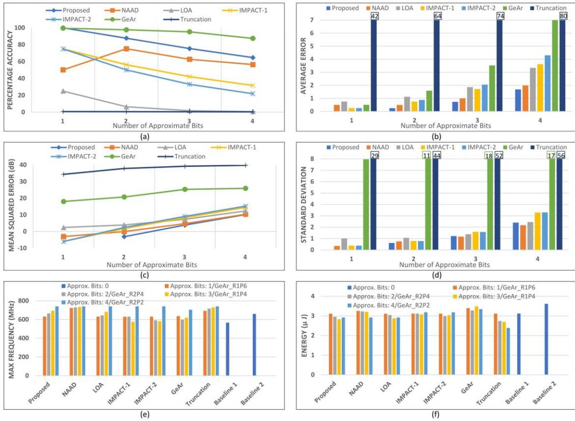
**Figure 2.7** Assessment Results (a) Percentage Accuracy (b) Average Error (c) Mean Squared Error (d) Standard Deviation (e) Maximum Frequency (f) Energy Consumption
