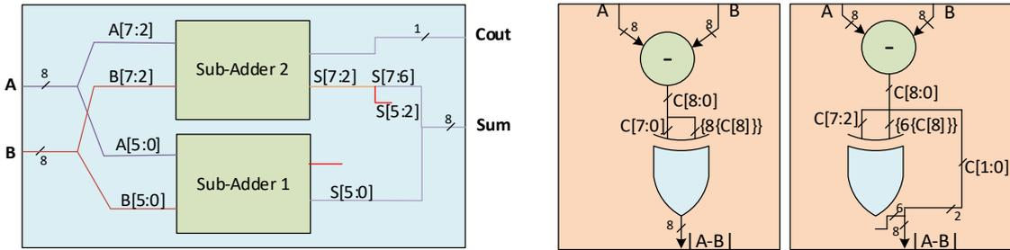
**Figure 2.5** (a) GeAr Adder ( $N=8, R=2, P=4$ ) (b) NAAD 0 (c) NAAD 2
