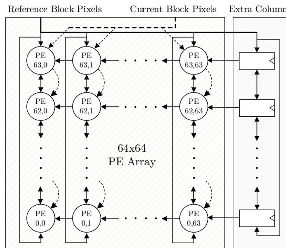
**Figure 3.5** Systolic processing element (PE) array and registers.
