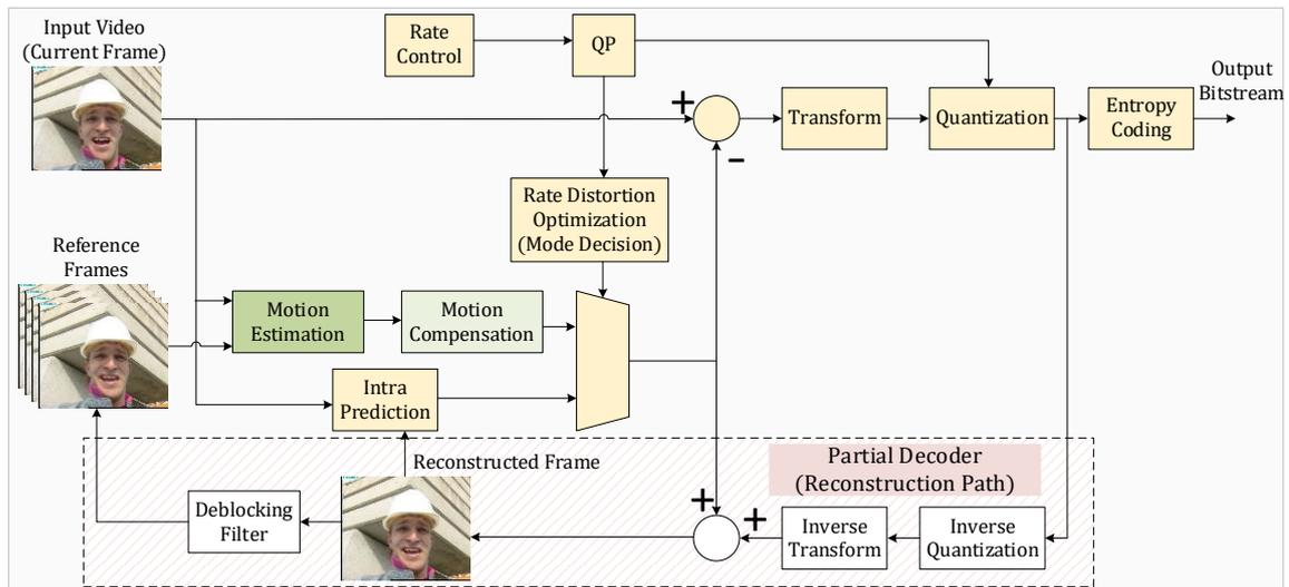
**Figure 1.5** Overview of a typical block-based encoder
