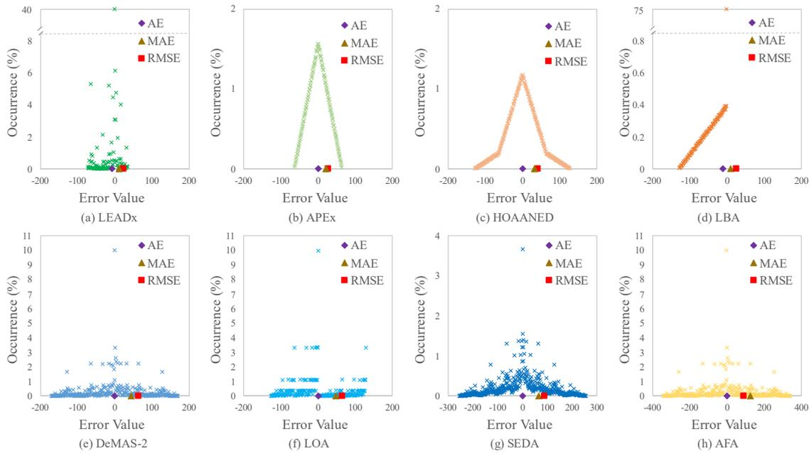
**Figure 5.8** Error distribution and error metrics of 16-bit approximate adders with 8-bit approximation.
