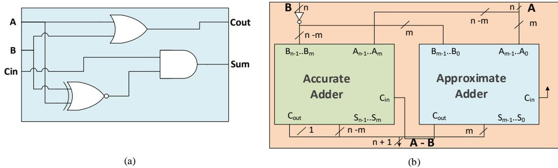
**Figure 2.2** (a) Proposed 1-bit Approximate FA (b)  $n$ -bit Approximate Subtractor
