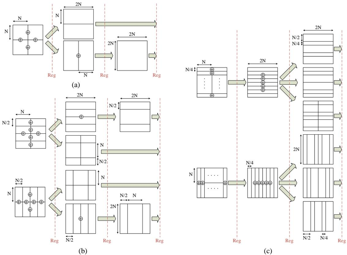
**Figure 3.9** SAD adder tree (a) SADs of BH, BV, Q partitions  $N = 4, 8, 16, 32$  (b) SADs of BH\_BH, BV\_TH, BH\_TV, BV\_BV, TH, TV partitions  $N = 8, 16$  (c) SADs of TH\_TH, TH\_BH, BH\_TH, BV\_TV, TV\_BV, TV\_TV partitions  $N = 16$ .
