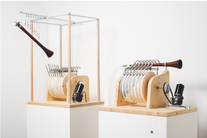
Figure 11: Recorder (left) player (right), Banu Musa's universal musical automaton , Baghdad ca. 850, re- built in 2015. Mikro-archaeological (re)construction team at Berlin University of the Arts:
