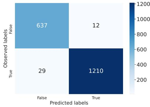
Figure B.4 Confusion matrix of XGBoost model with mean and variance features to detect machine imbalance with input length of 5 seconds
