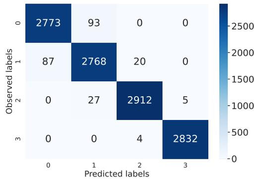
Figure B.9 Confusion matrix of XGBoost model with DFT features to detect load imbalance with input length of 1 second
