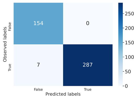
Figure B.6 Confusion matrix of SVM model with mean and variance features to detect machine imbalance with input length of 20 seconds
