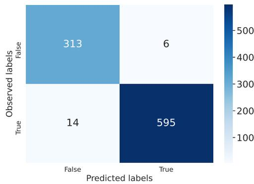
Figure B.5 Confusion matrix of XGBoost model with mean and variance features to detect machine imbalance with input length of 10 seconds
