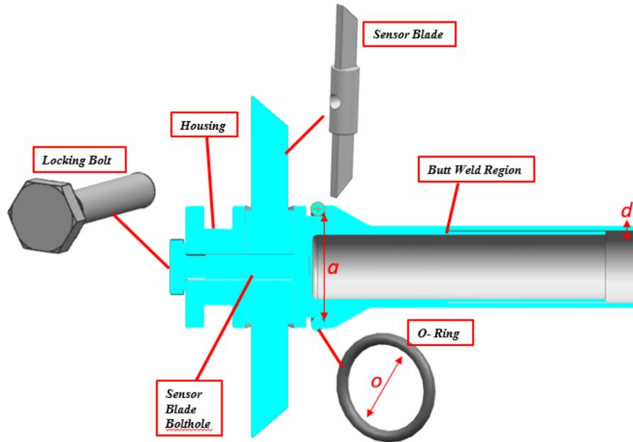
Figure 15 3D Model and Cross Section of the Torquemeter Front Side
