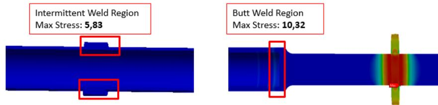
Figure 28 Equivalent Stresses on Welding Joints-2
