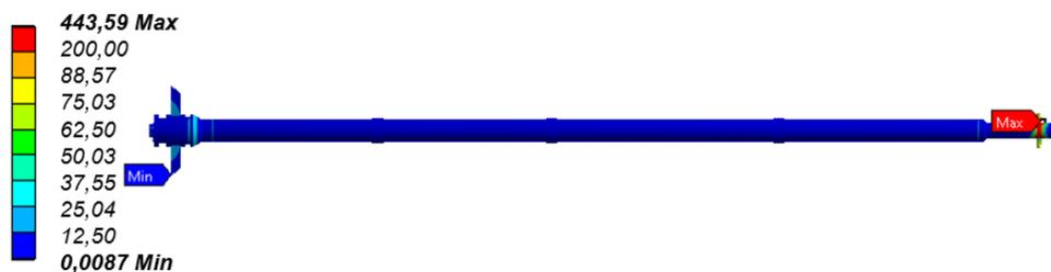
Figure 23 Max and Min Equivalent Stresses on Torquemeter
