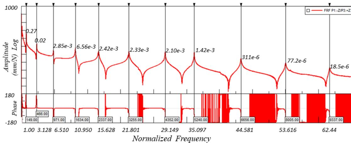
Figure 35 Amplitude and Phase of a FRF Function
