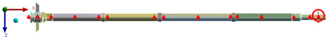
Figure 32 Accelerometer Location and Measurement Points
