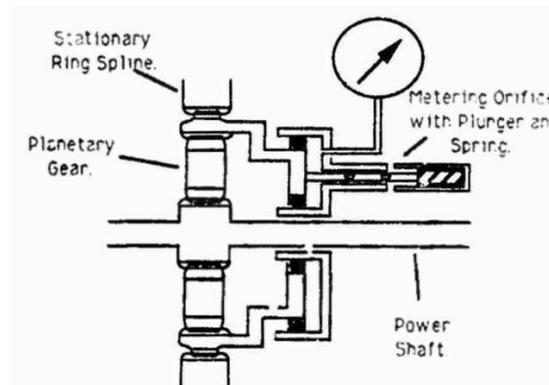
Figure 3. Hydromechanical torque measurement unit (AGARD, 1994)
