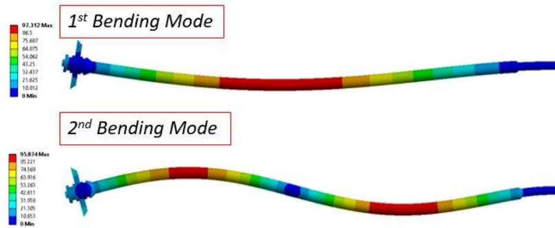
Figure 29 Mode Shapes for Middle Rings Location
