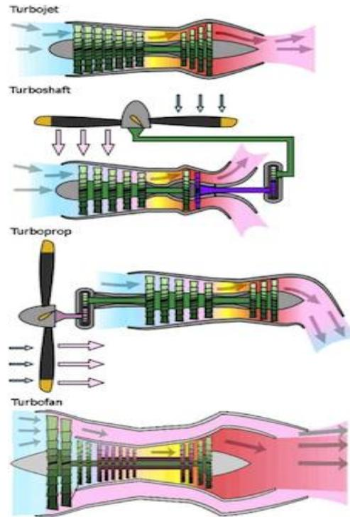
Figure 2. Types of Gas Turbine Engines (*Hünecke, 1997*)
