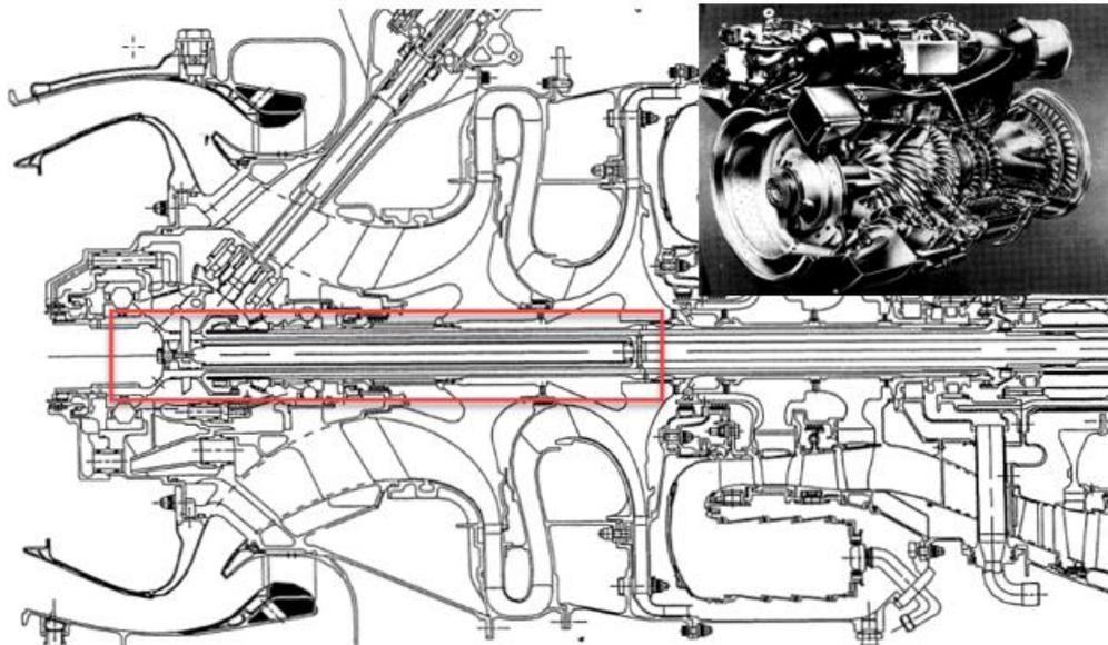
Figure 11. LHTEC T800 Turboshaft Engine (Becker & Frounfelker, 1992)
