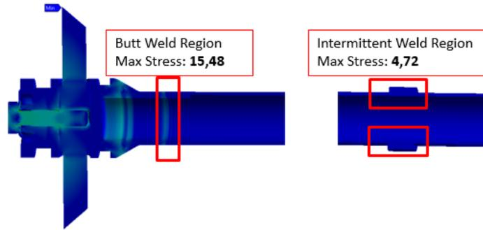
Figure 27 Equivalent Stresses on Welding Joints-1
