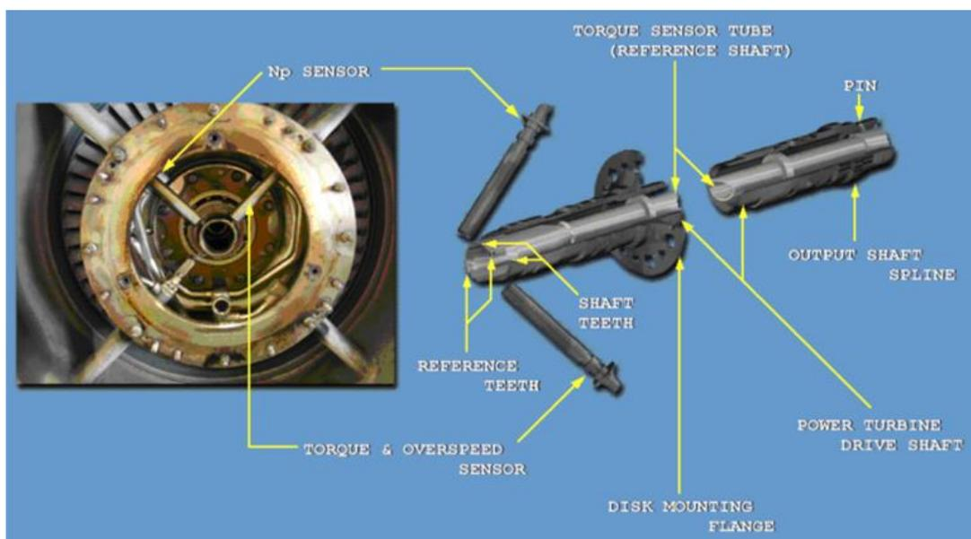
Figure 9. T700 Turboshaft Engine Torque Measurement Unit (*US Army Aviation, 2007*)
