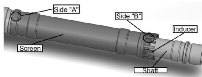
Figure 7. 3D model of torque measurement unit, Motor Sich (Sirenko, Yepifanov, Podgorsky, & Nechunaev, 2018)
