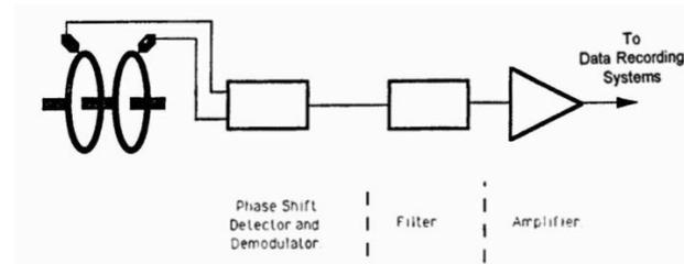
Figure 5. Angular twist torque measurement unit (AGARD, 1994)
