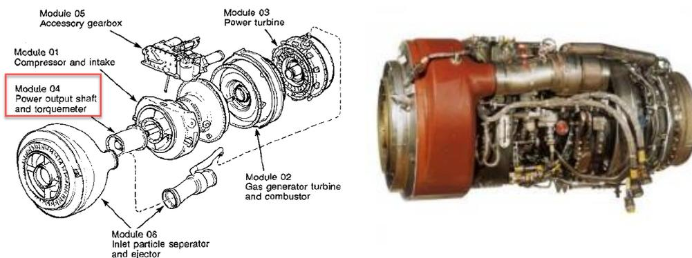
Figure 10. RTM 322 Turboshaft Engine Layout (Lewis & Buller, 1985), (Engines, 2020)
