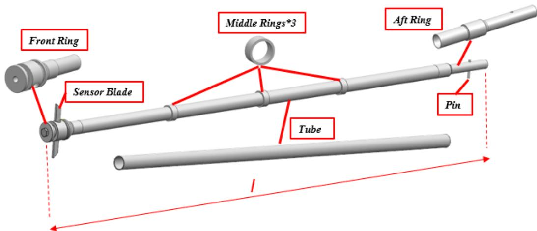
Figure 14 3D Model of Torquemeter (Reference Shaft)
