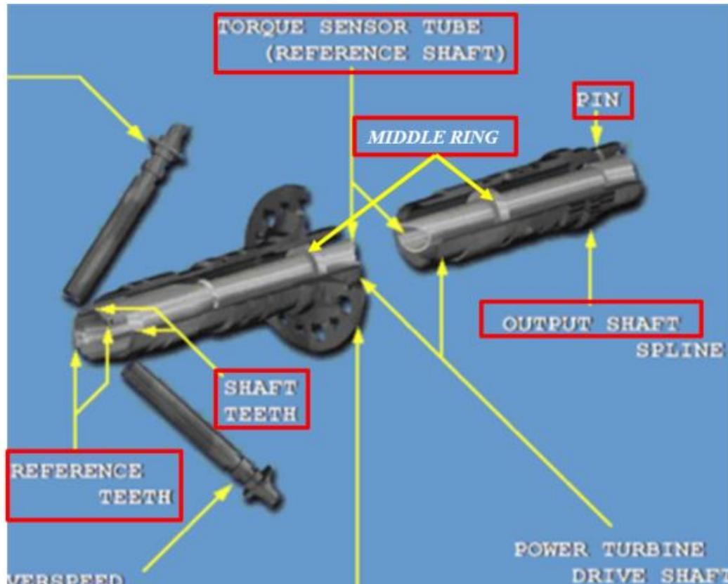
Figure 13 T700 Reference Shaft Geometry (*US Army Aviation, 2007*)
