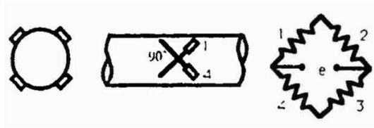
Figure 4. Strain-gauge torque measurement unit (US Patent No. 7698959, 2010)
