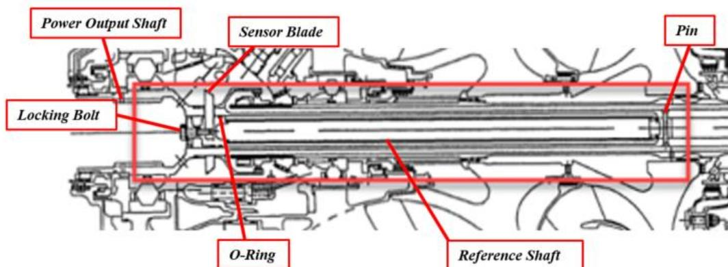
Figure 12 T800 Reference Shaft Geometry (*Becker & Frounfelker, 1992*)
