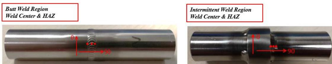
Figure 26 Test Specimen for XRD Measurement
