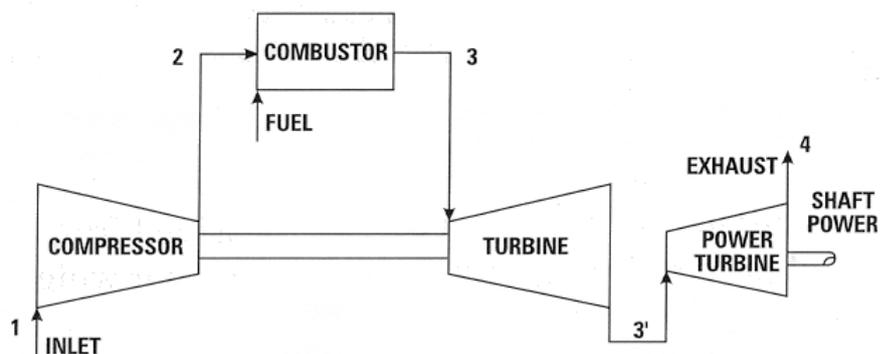
Figure 1. Mechanical arrangement of a gas turbine engine
