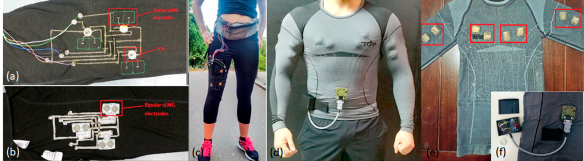
Figure 3.4 Wearable electromyography (EMG) acquisition garments: running leggings and a sports shirt. Electrode placement in the (a) exterior; and (b) interior of leggings; (c) actual view of leggings when worn by a subject [16] ;(d) shirt as worn by a subject; (e) location of electrodes on the shirt; (f) close-up view of the acquisition unit attached to the shirt [58].
